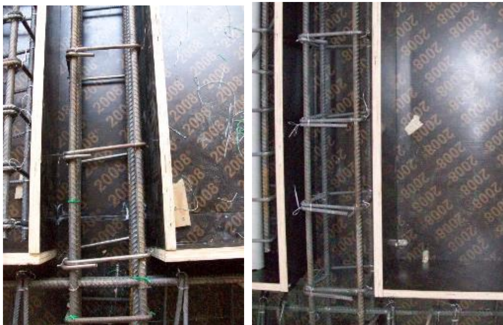
Figure 3.5. Specimen with plain stirrup steel (left) and specimen with deformed stirrup steel (right)
