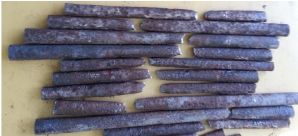
Figure 3.2. Naturally corroded test specimen
