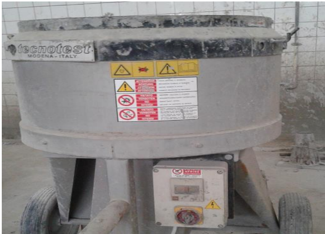
Figure 3.4: Concrete Mixer (0.25) m 3 Capacity
