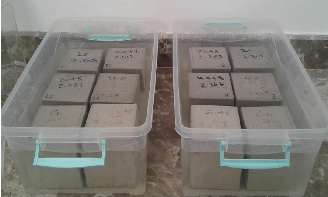
Figure 3.11: Samples in Sulphate Solution
