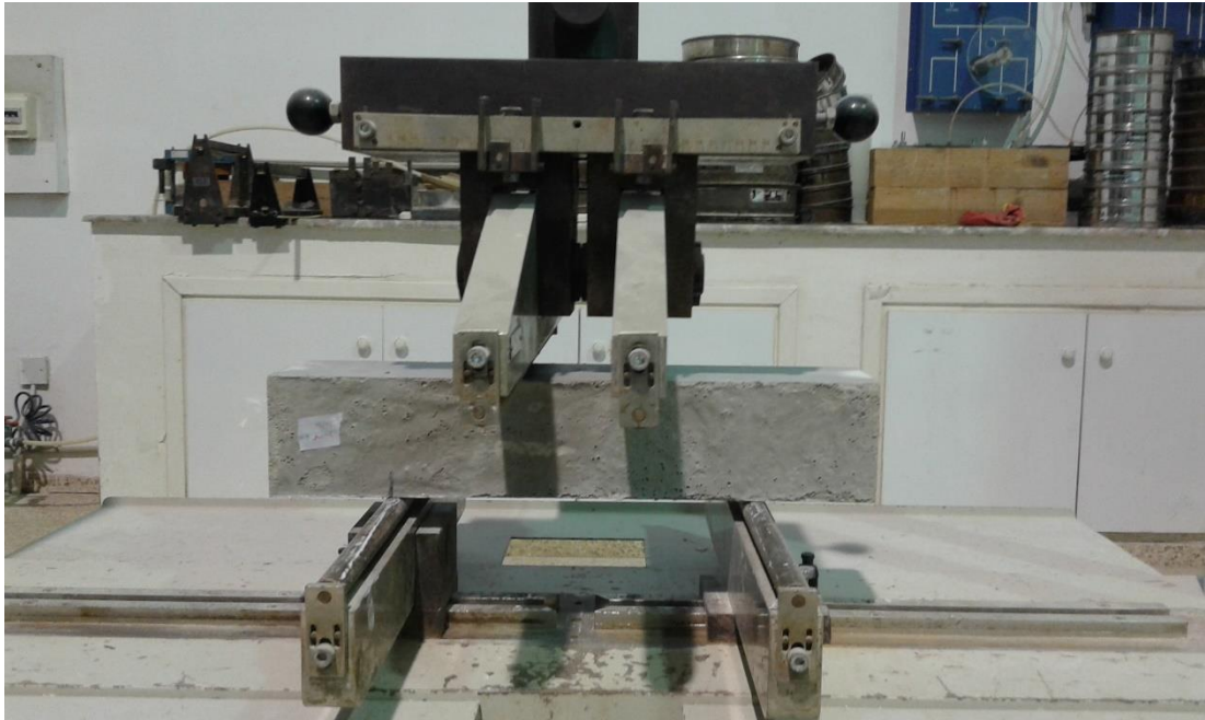
Figure 3.9: Flexural Strength Testing
