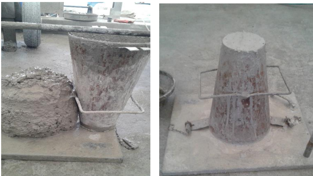
Figure 3.7: Slump Test for Workability
