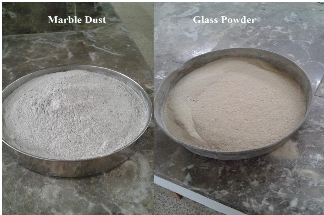
Figure 3.3: Marble Dust and Glass Powder
