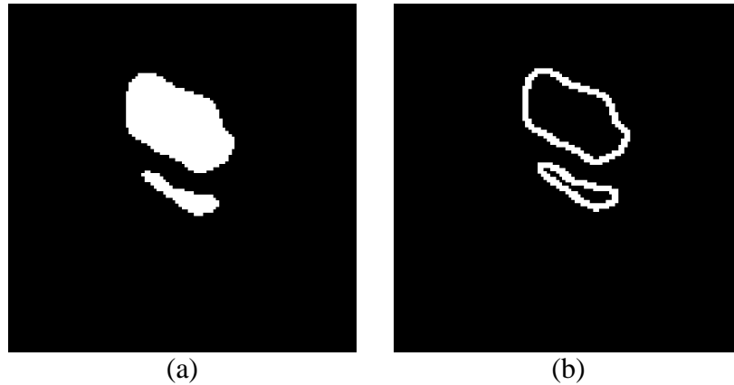
Figure 3.11: The procedure of produce boundary from area for combined target-shadow region a. TSA, b. TSB
