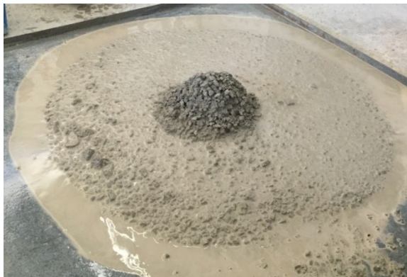
Figure 25: Bleeding and segregation in slump-flow test of SS10SP2
