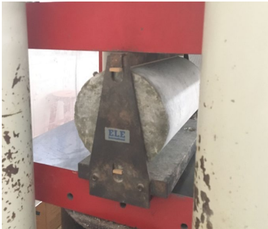
Figure 16: Placement of cylindrical specimen in aligning jig for splitting tensile strength
