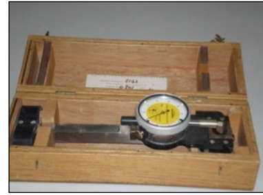
Figure 22: Demec positions on the cubes and Demec Gauge instrument
