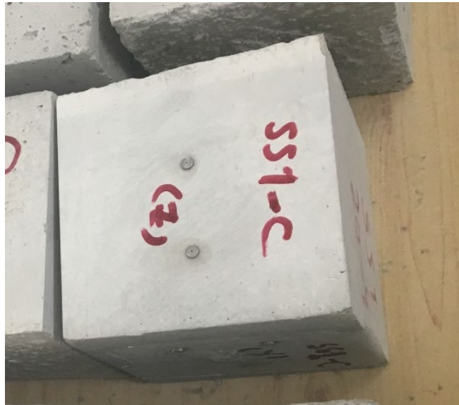
Figure 23: SS specimen with pins in three directions for volume change measurement
