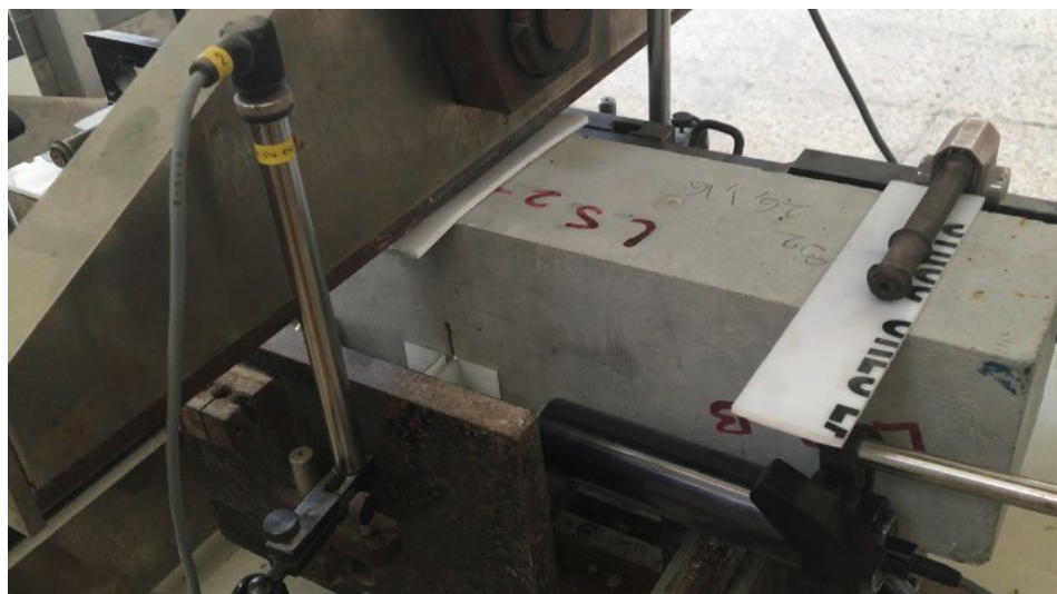
Figure 21: Notched beam under TBT test
