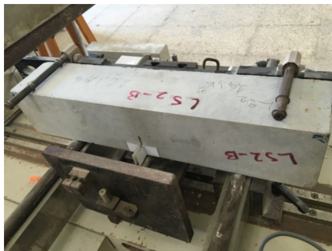
Figure 20: Prismatic beam prepared for fracture energy test with 40 mm notch
