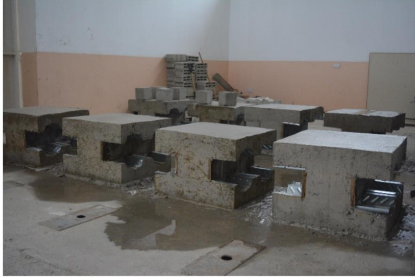
Figure 3.16: Slip capacity specimens during curing process.
