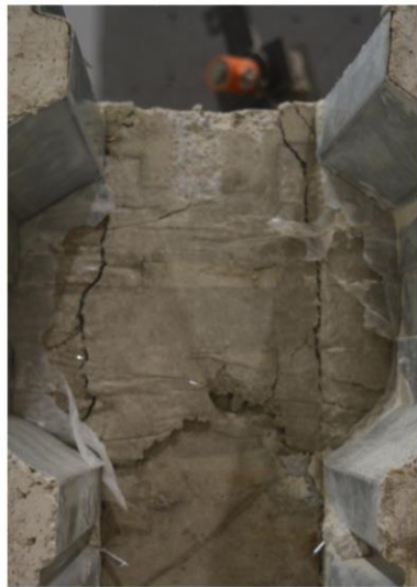
Figure 4.29: Local shear between the slabs and the beam specimen series of SC-SR.
