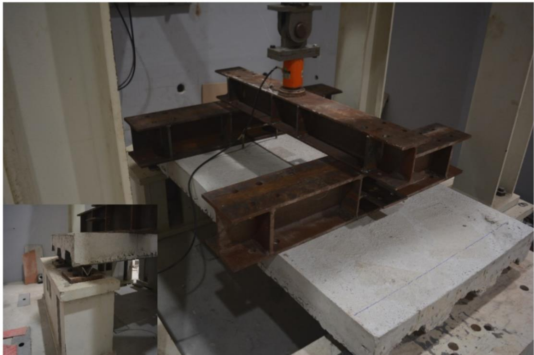
Figure 3.10: Load set-up for m-k test short span specimen.
