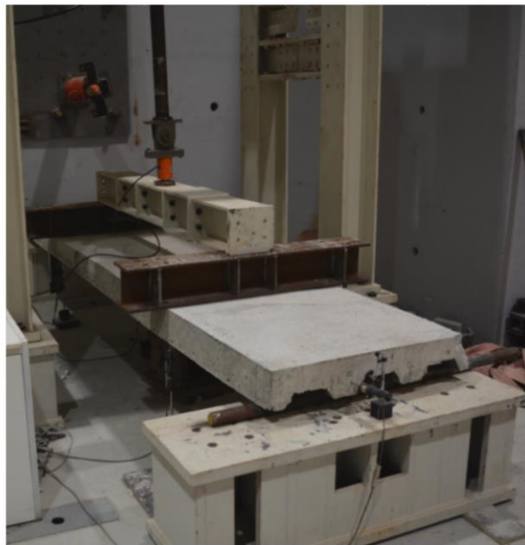
Figure 3.12: Load set-up for m-k test long span specimens.
