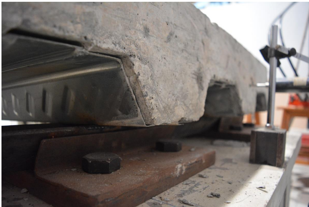
Figure 4.21: End-slip after failure for specimen mk-LS1s.
