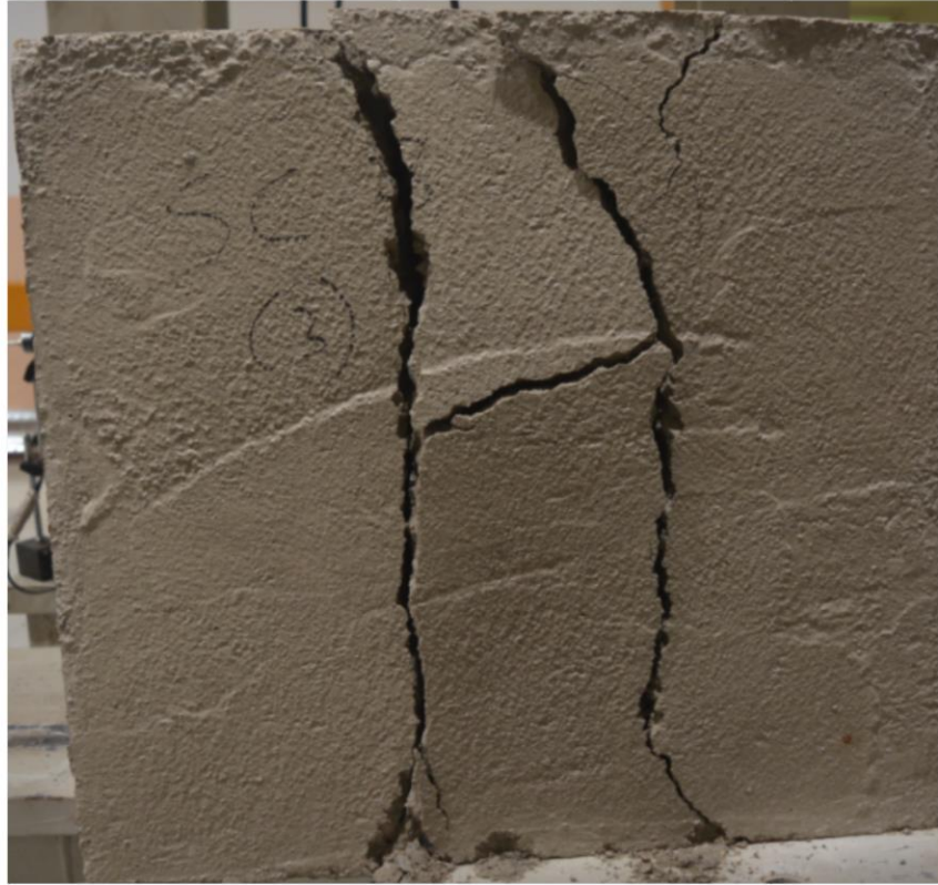
Figure 4.33: Mode of failure for specimen series of SC-Con.
