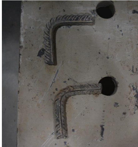
Figure 4.35: Shape of connector after failure specimen series of SC-Con.
