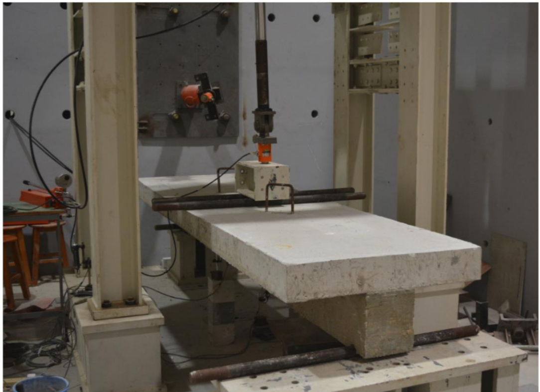
Figure 3.6: Static test load set-up for RC T-beam.
