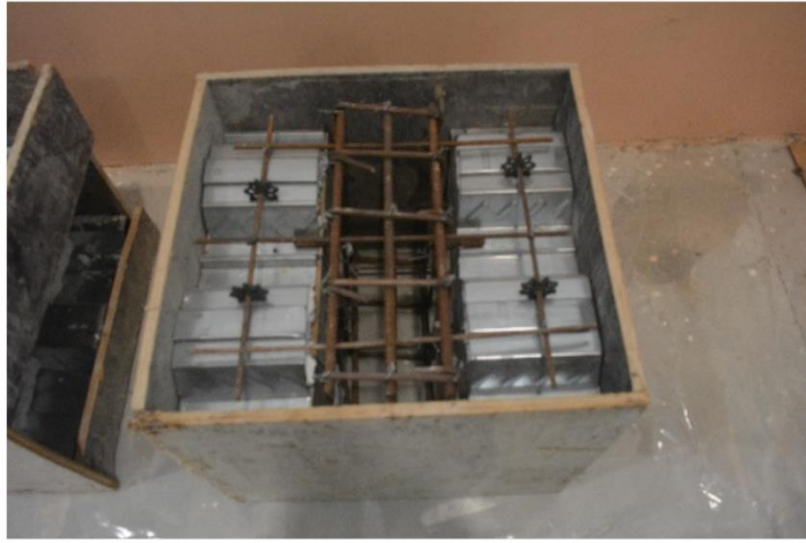
Figure 3.14: View of slip capacity specimen before concreting.
