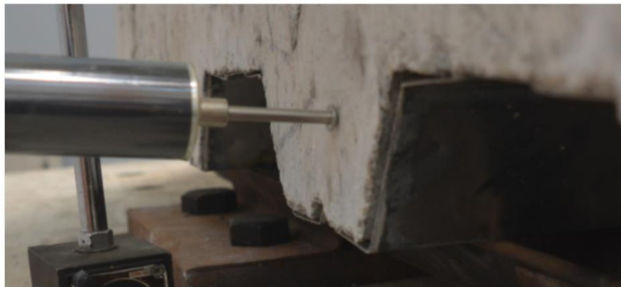
Figure 4.13: Beginning of end-slip during the test process.
