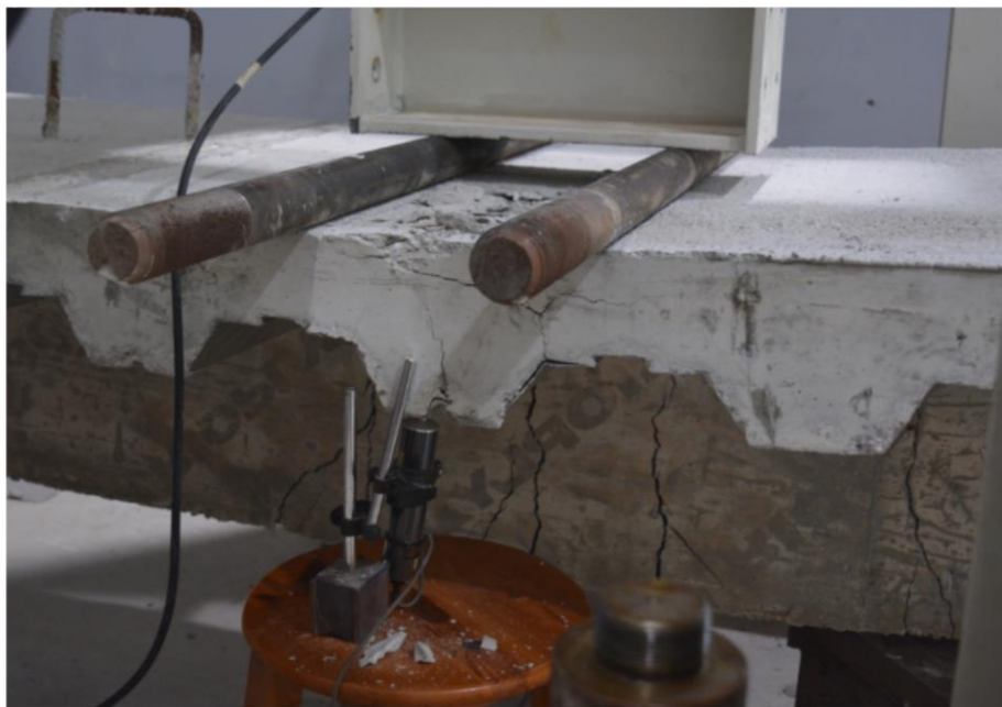
Figure 4.3: Longitudinal shear of the slab in the zone of pure-bending at the failure load of specimen CS.
