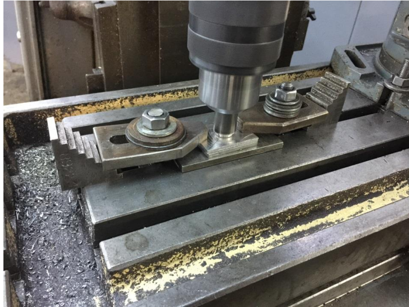
Figure 15: Lap-joint configuration of dissimilar Al-Ti alloys
