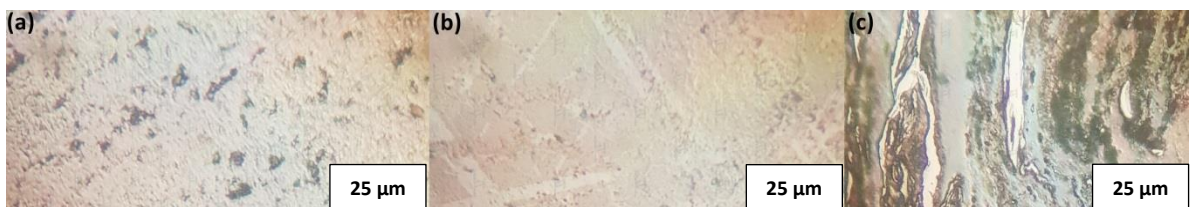
Figure 36: (a) Microstructure of Sample 1, Ti cross-section (a) BM, (b) HAZ and (c) TMAZ. . Photomicrograph was taken via metallurgical microscope
