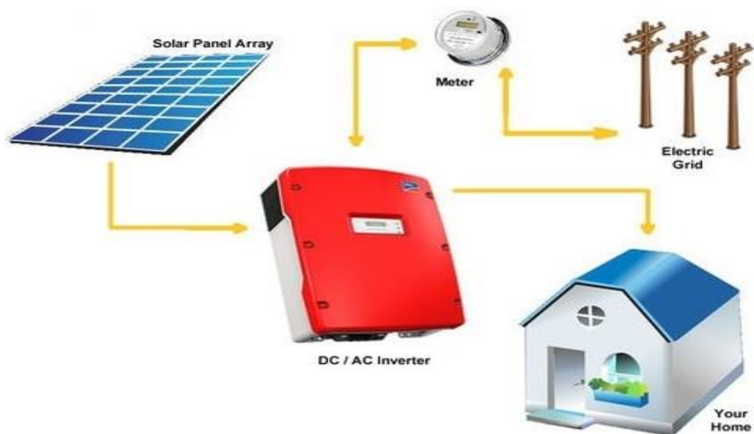
Figure 3: The schematic diagram of an on-grid system (Alfadhli, et al., 2019).
