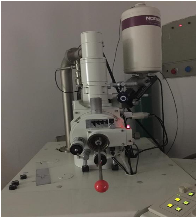
Figure 3.8: JEOL JSM-6400 Equipped with a NORAN System 6 X-Ray Microanalysis System
