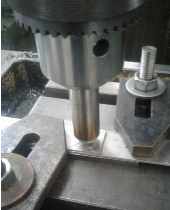
Figure 3.4: Clamping fixture mechanism utilized during FSSW
