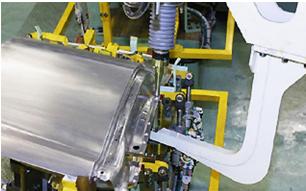
Figure 2.7: Mazda Aluminum joining Technology by FSSW (Mazda, 2003)
