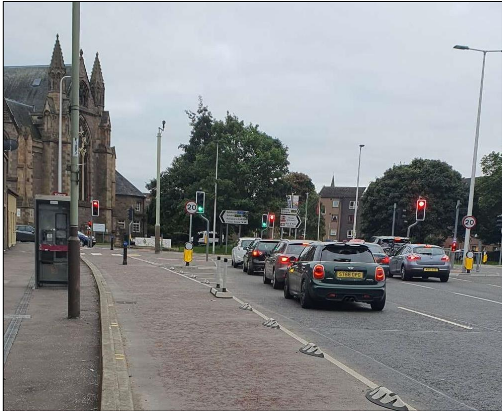
Figure 51: Example of Cycle Lane Soft Segregation
