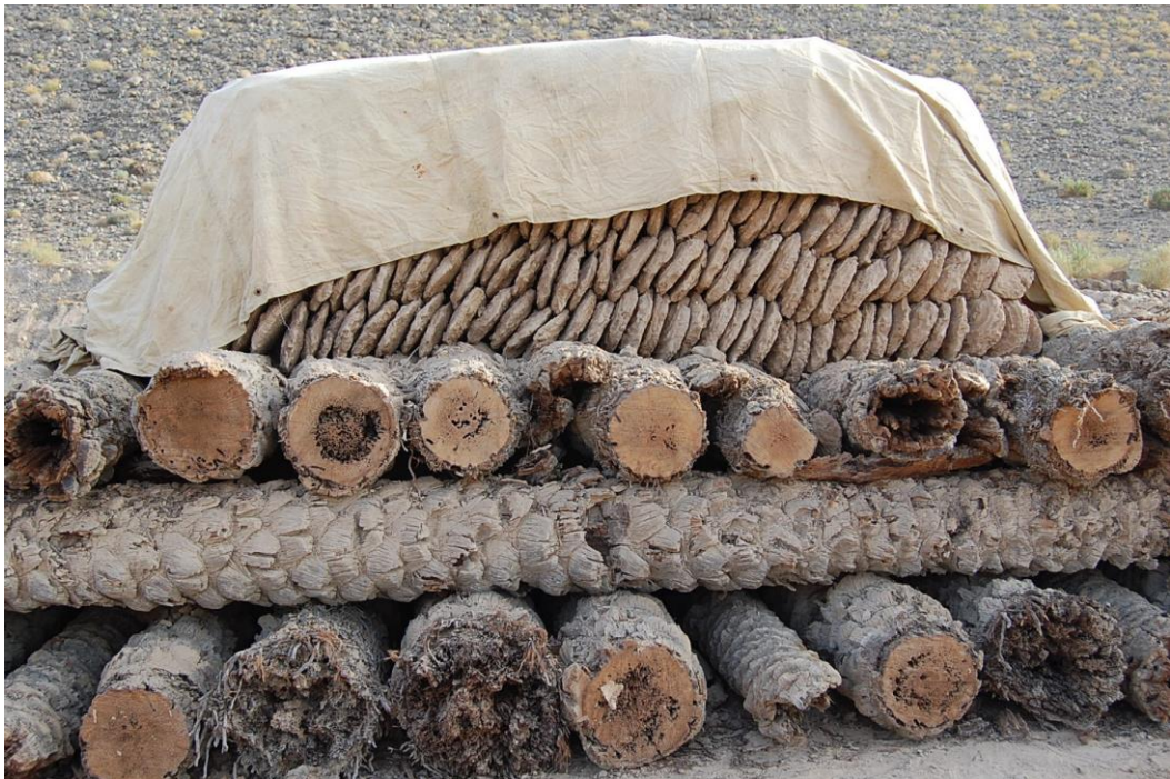
Figure 19: Saruj Preparation – The discs are burned on layers of palm trunks. [Photograph]. Copyright 2007 by Emirates Natural History Group
