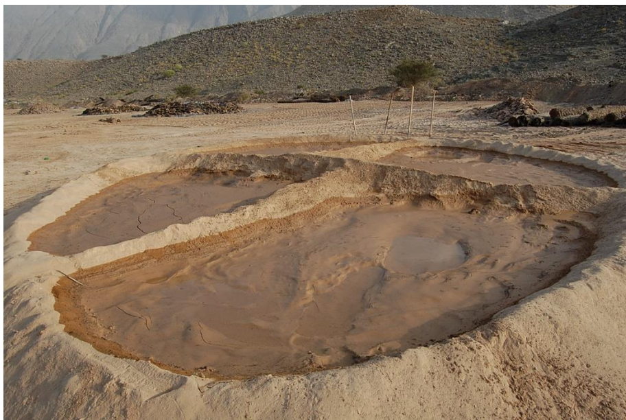
Figure 17: Saruj preparation - Soaking of raw material [Photograph]. Copyright 2007 by Emirates Natural History Group
