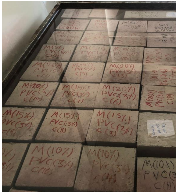
Figure 13: Curing water tank.
