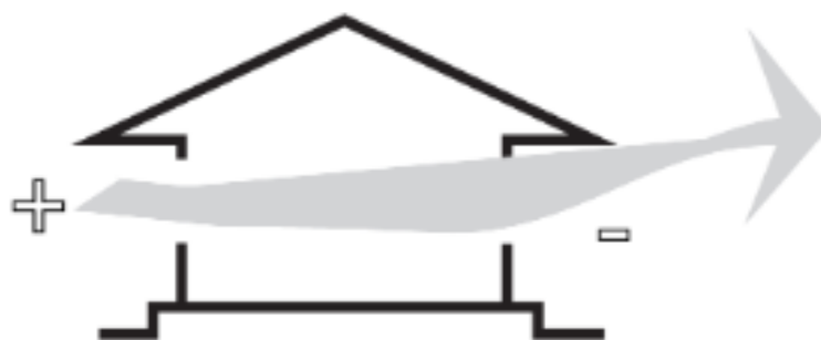
Figure 10: Wind Effect Principle Work. Source: (Faggianelli et al., 2013)
