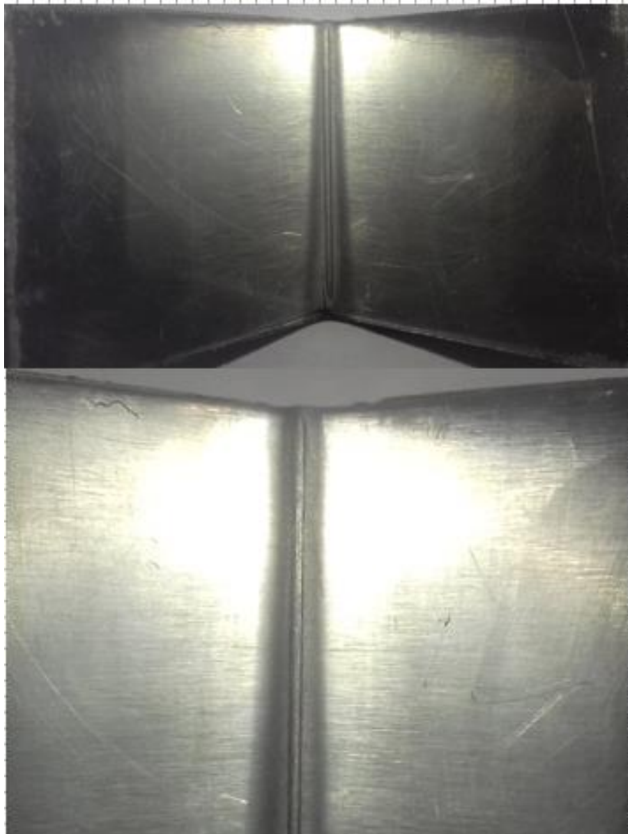
Figure 3.6c: Bend Specimen Viewed under x 30 Magnification: Interior
