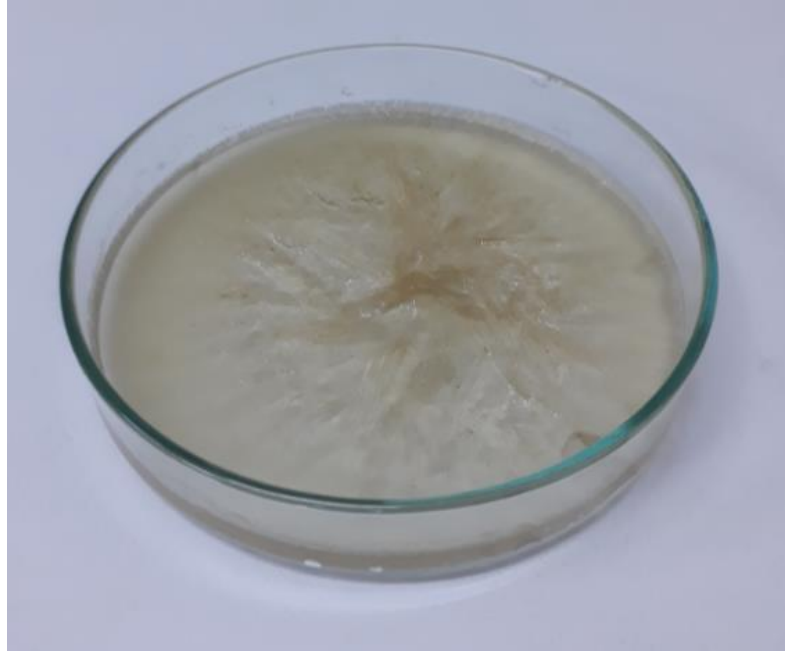
Figure 6: Cryogel sample after freeze thawing process
