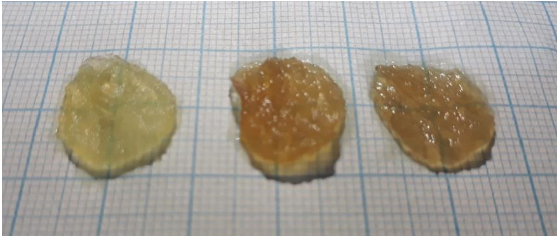
Figure 7: Indication of silver nanoparticle formation as a result of colour change (left: no silver, middle: 0.01M 10mL silver nitrate, right: 0.1M 1mL silver nitrate)
