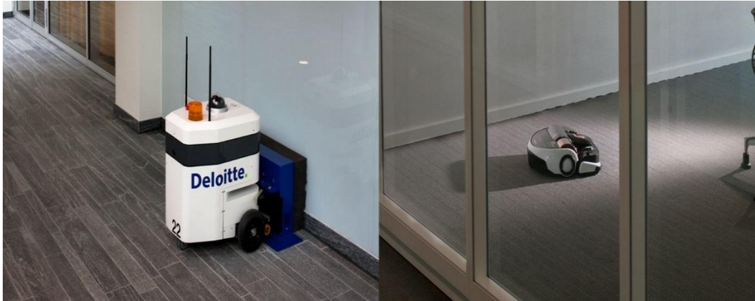
Figure 2.8: The Cleaner and Security Robots of the Edge Building (Bloomberg, 2015)
