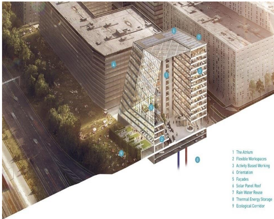
Figure 2.7: Different Part of the Edge Building (Build Up, 2017)
