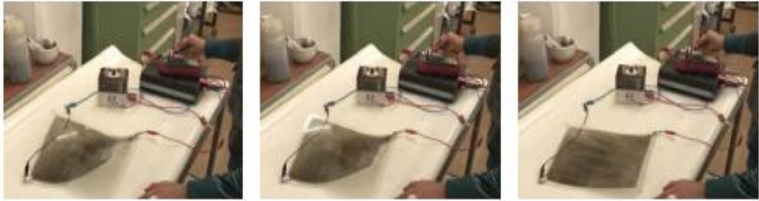
Figure 3.15: ShapeShift can Changes its Size, Shape and Volume Through High Voltage of Electricity (Fox, 2016)
