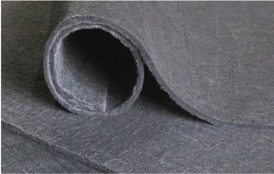
Figure 3.6: Aerogel Blankets (ProctorGroup,2019)
