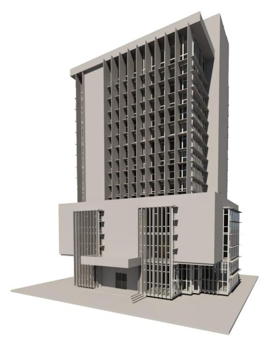
Figure 57: 3D View of Egg-Crate Shading System at the West Façade (Author, 2021)
