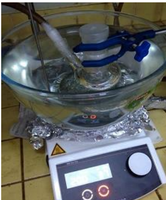
Figure 2.1. The grafting reaction preparation under nitrogen atmosphere
