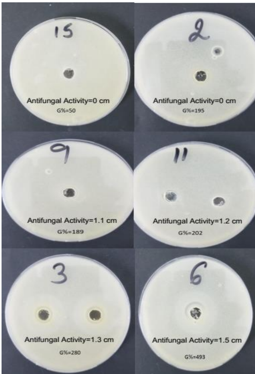
Figure 2.16. Antifungal analysis of pullulan- graft -NVI samples with grafting yields of (50%, 195%, 189%, 202%, 280%, 493%) against Candida albicans fungi
