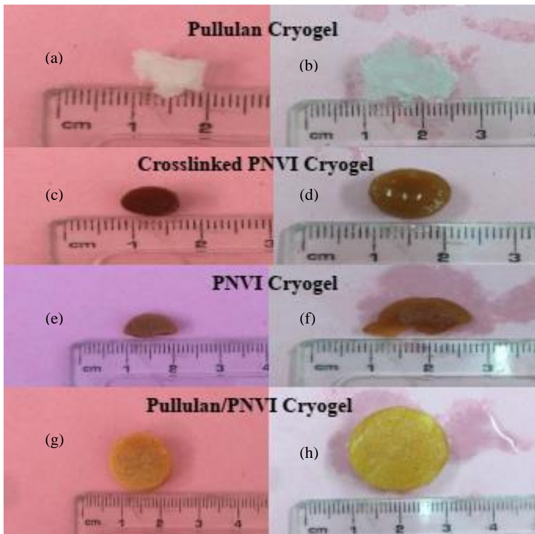
Figure 4.22. (a) Freeze dried pullulan cryogel, (b) swollen pullulan cryogel, (c) freeze dried crosslinked PNVI cryogel, (d) swollen crosslinked PNVI cryogel, (e) freeze dried PNVI cryogel, (f) swollen PNVI cryogel, (g) freeze dried pullulan/PNVI cryogel, (h) swollen pullulan/PNVI cryogel
