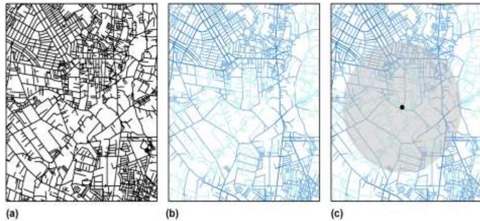
Figure 34: The procedure of computing space syntax measures: (a) base map (street centerlines); (b) space syntax measure of integration considered for each street segment, (c) area-level measures calculated by combining integration values in a buffer zone (Koohsari et al., 2019)
