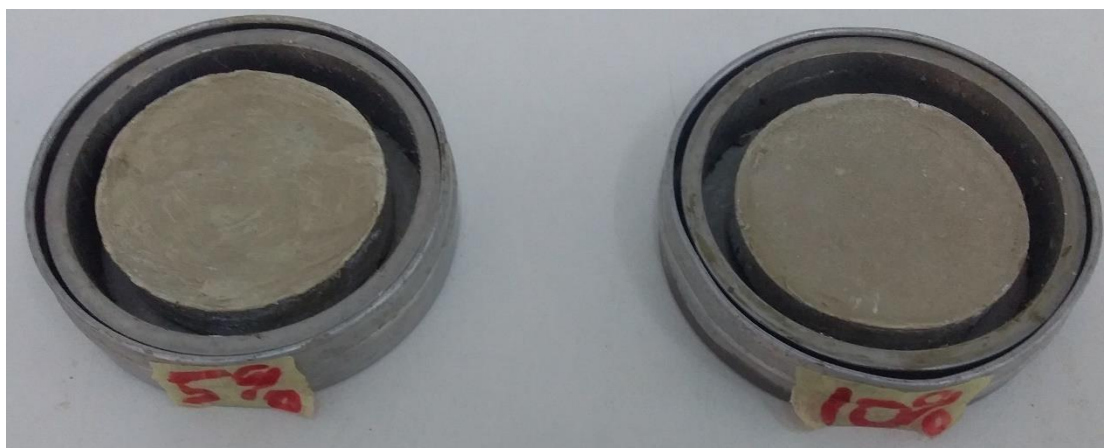
Figure 4.6: Soil Specimen with 5% and 10% Bentonite After Oven-drying
