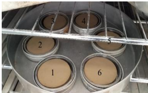
Figure 3.9: Soil Specimen for Desiccation Cracks During Oven-drying
