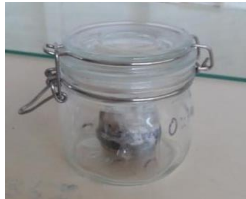
Figure 3.7: Soil Specimen Placed in a Jar
