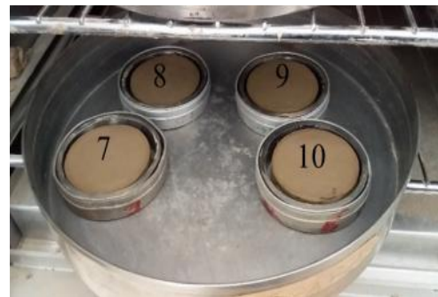
Figure 3.9: Soil Specimen for Desiccation Cracks During Oven-drying
