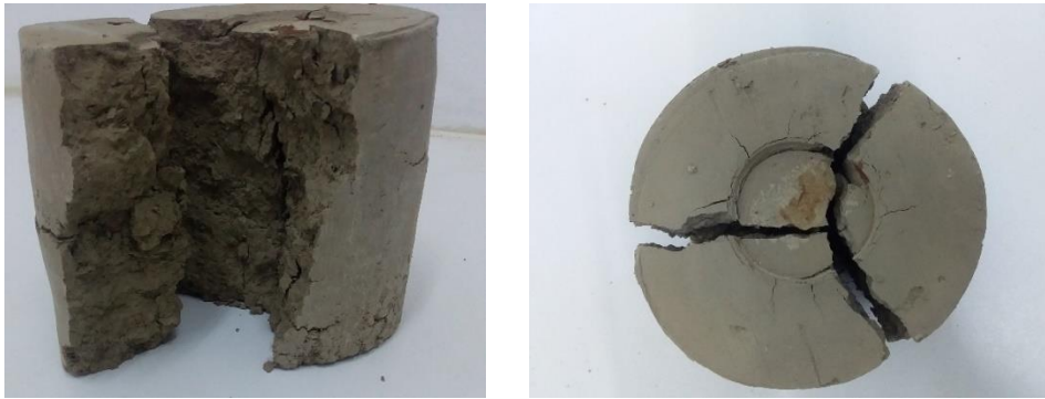
(a) (b) Figure 4.16: Double Punch Test: (a) Sample After Failure (b) Radial Tension Cracks
