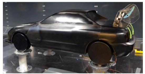
Figure 1: 1:25 scale Honda CR-X del Sol model from the study of Kurec et al [7].
