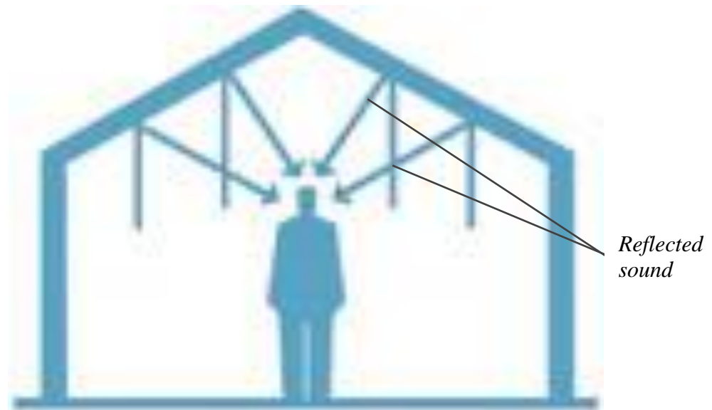
Fig. 2.11: Reflection Illustration (Adapted from Harris, 1994)
