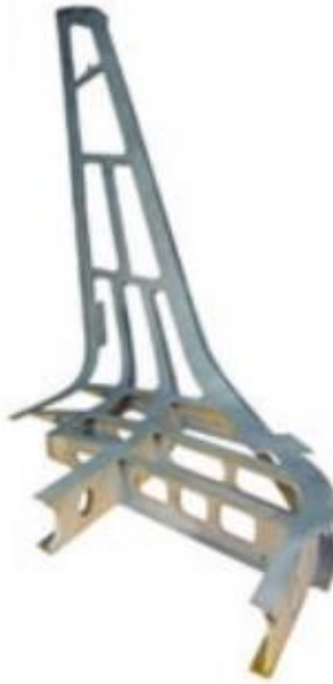
Figure 2.5: Winglet Substructure of Embraer Phenom by using F357 Alloy that is made in the Investment Process [5]
