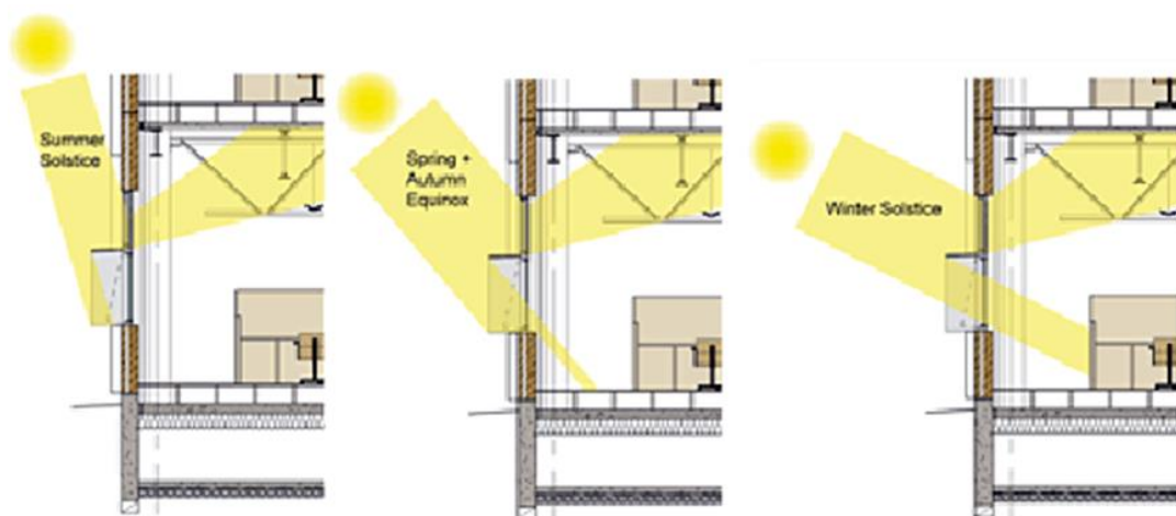
Figure 29. Seasonal performance of shading, redirection devices (URL 3. www.liamd.pw , 2019)
