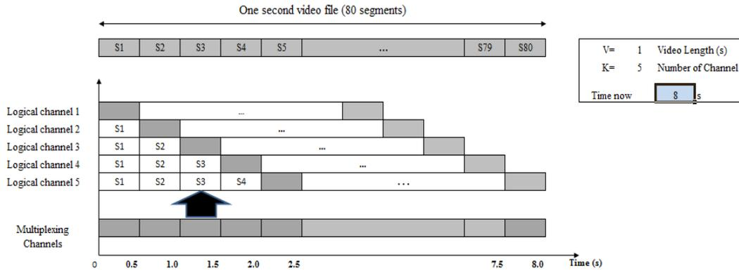
Figure 25: Multiplexing channel/multicast, time= 8 s
