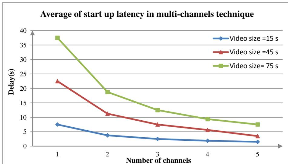
Figure 40: Effects of multi-channeling/multicast on start up latency
