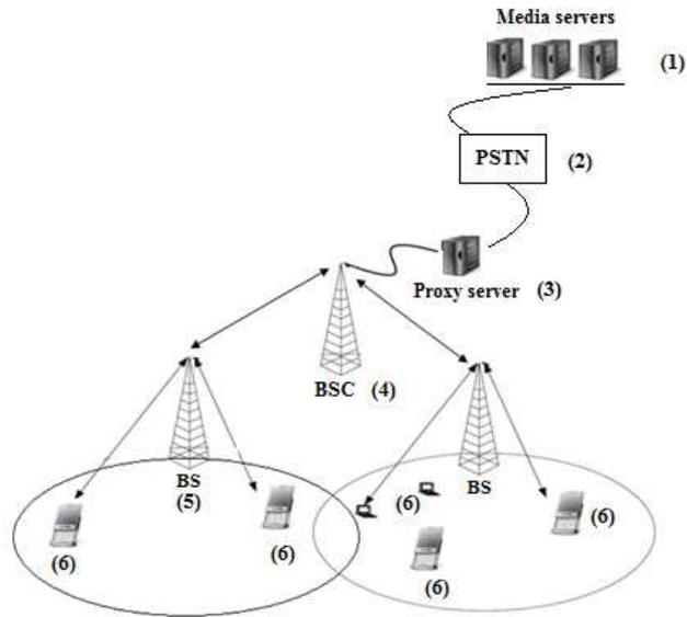
Figure 16: Architecture of Proposed System
