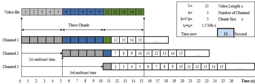
Figure 28: Multi-channel/multicast implementation (3rd multicast started, time=11 s)
