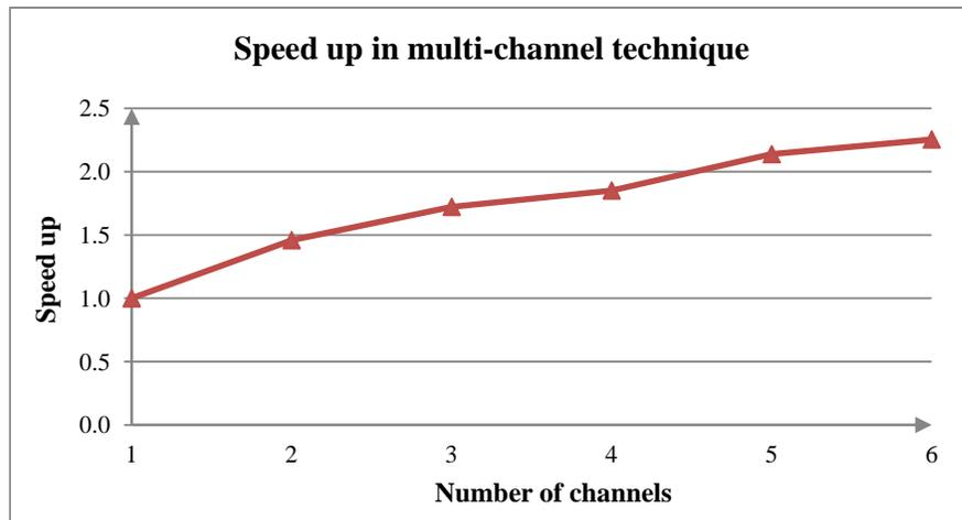
Figure 42: Speeds up in multi-channeling
