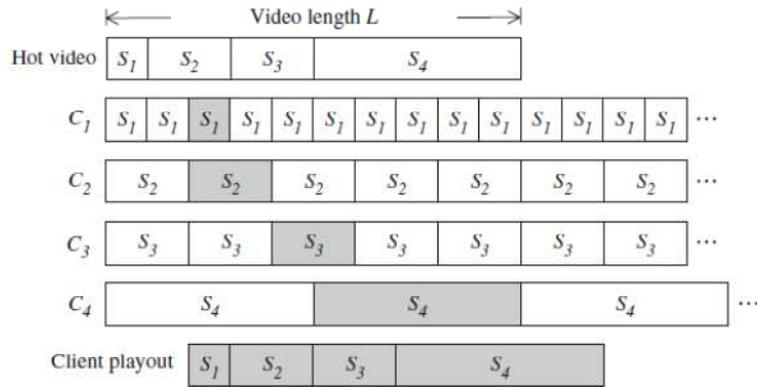
Figure 2: Illustration of segment downloading for the SkB technique, where number of channels is  $k=4$ , [19]
