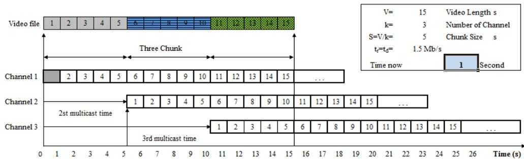
Figure 26: Multi-channel/multicast implementation (1st multicast, time = 1 s)
