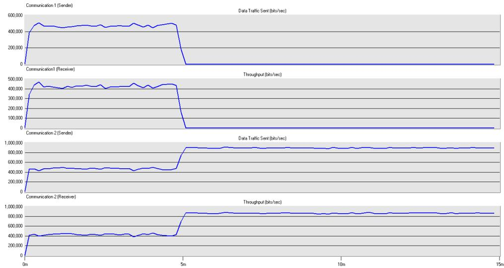
Figure 36: Effect of interferences in wireless communication
