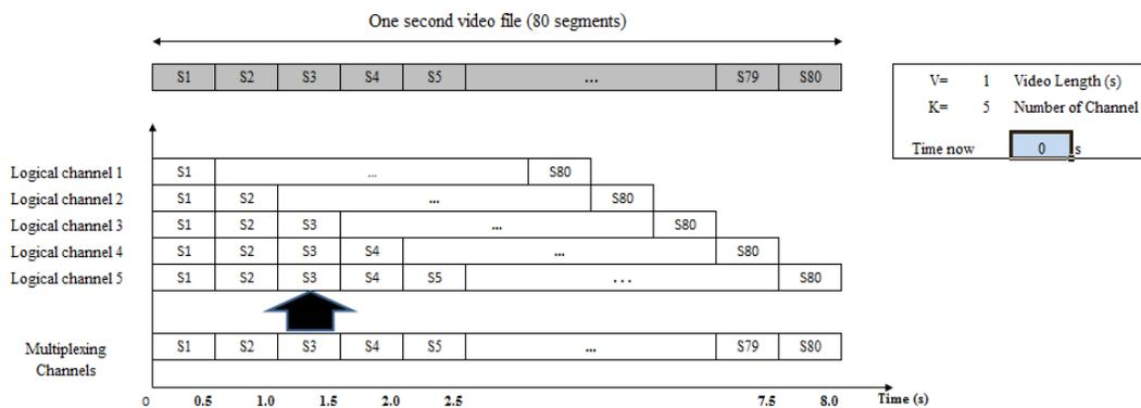
Figure 21: Multiplexing channel/multicast, time= 0.0 s
