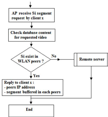
Figure 14: AP side diagram for WLAN function
