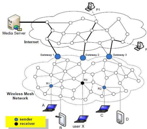
Figure 4: VoD in Wireless mesh networks [11]
