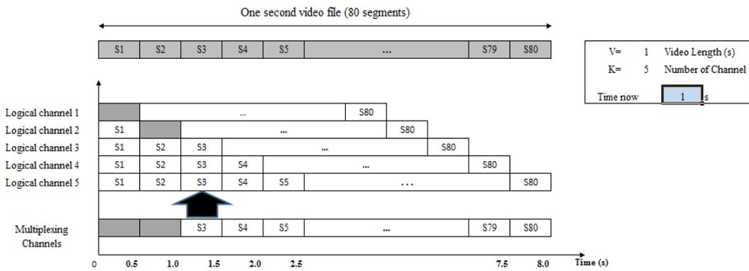
Figure 23: Multiplexing channel/multicast, time= 1 s
