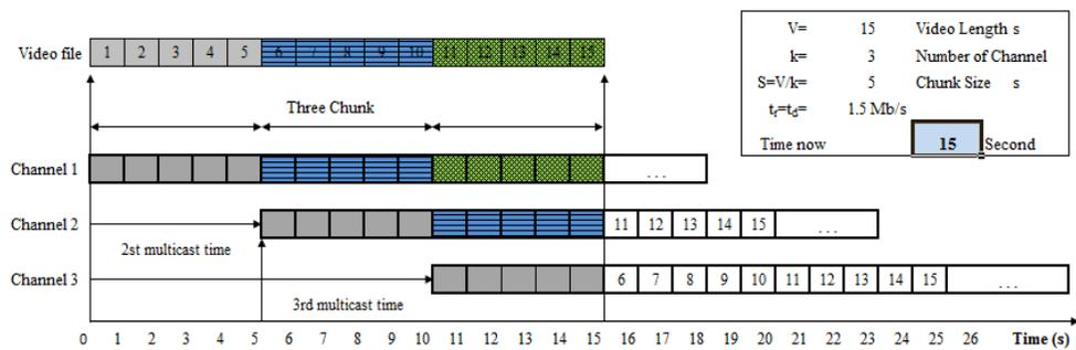
Figure 29: Multi-channel/multicast implementation (1st multicast finished, time=15s)
