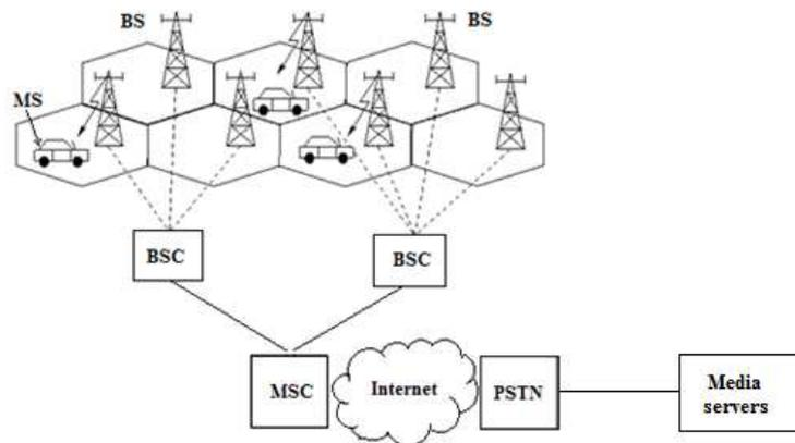
Figure 6: Architecture of a cellular wireless network
