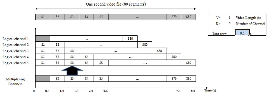
Figure 22: Multiplexing channel/multicast, time= 0.5 s
