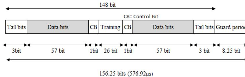
Figure 10: Functions of the bits in normal transmission burst.
