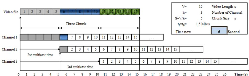
Figure 27: Multi-channel/multicast implementation (2nd multicast started, time=6 s)
