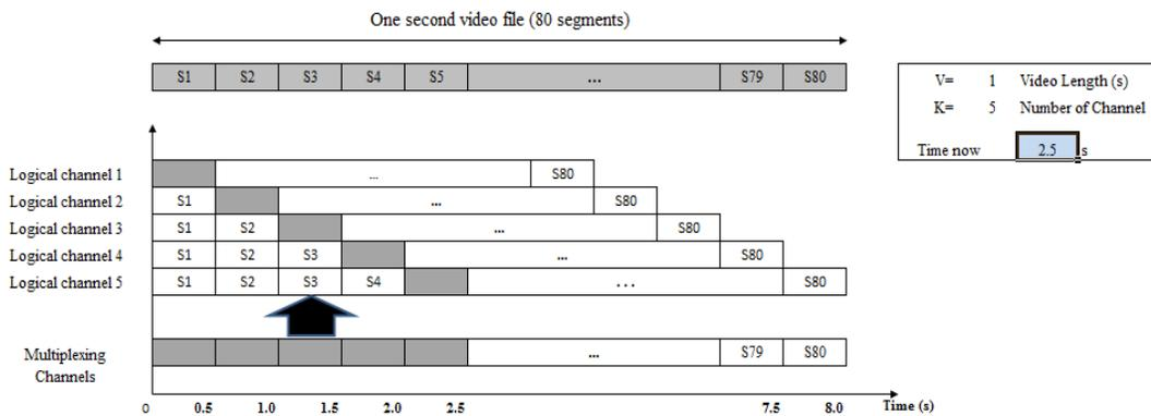
Figure 24: Multiplexing channel/multicast, time= 2.5 s
