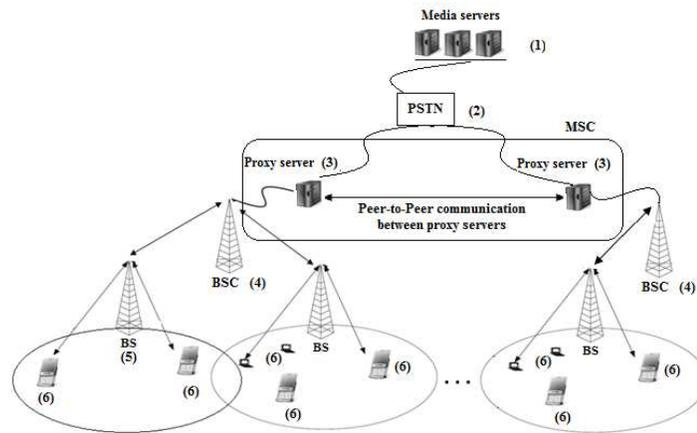
Figure 44: Peer-to-Peer communication based proxy server
