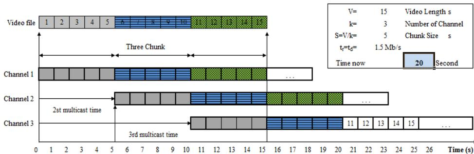
Figure 30: Multi-channel/multicast implementation (2nd multicast finished, 3rd multicast continuing, time=20s)
