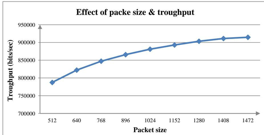
Figure 39: Effect of packet size and throughput
