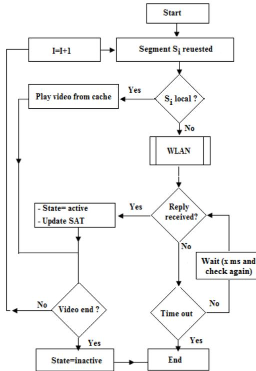
Figure 13: Client side function for requested video by WLAN clients
