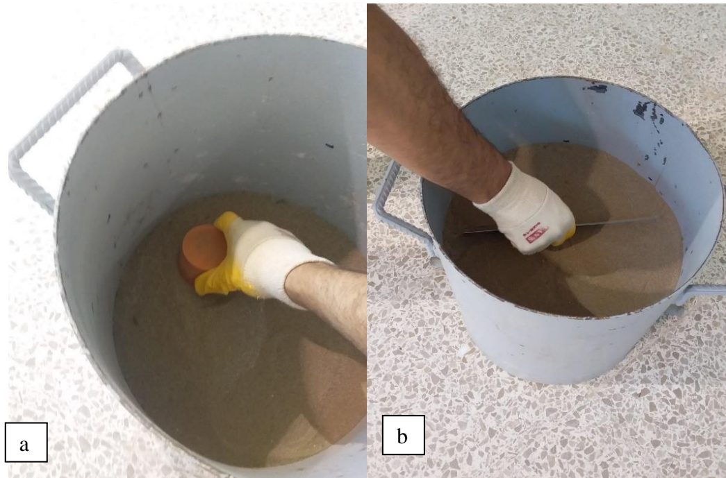
Figure 3.14: Placement of the sand in the test tank: (a) compacting sand in the test tank (b) levelling the surface of the sand
