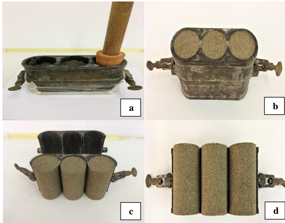
Figure 3.11: Specimens compaction and extraction processes in the mold: (a) compacting the mixture, (b) trimmed surface of the specimens, (c) splitting the mold, (d) extracting the specimens
