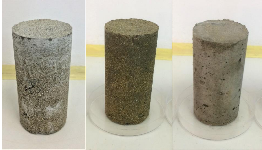
Figure 3.8: Specimens prepared with different water–binder ratios, W/B
