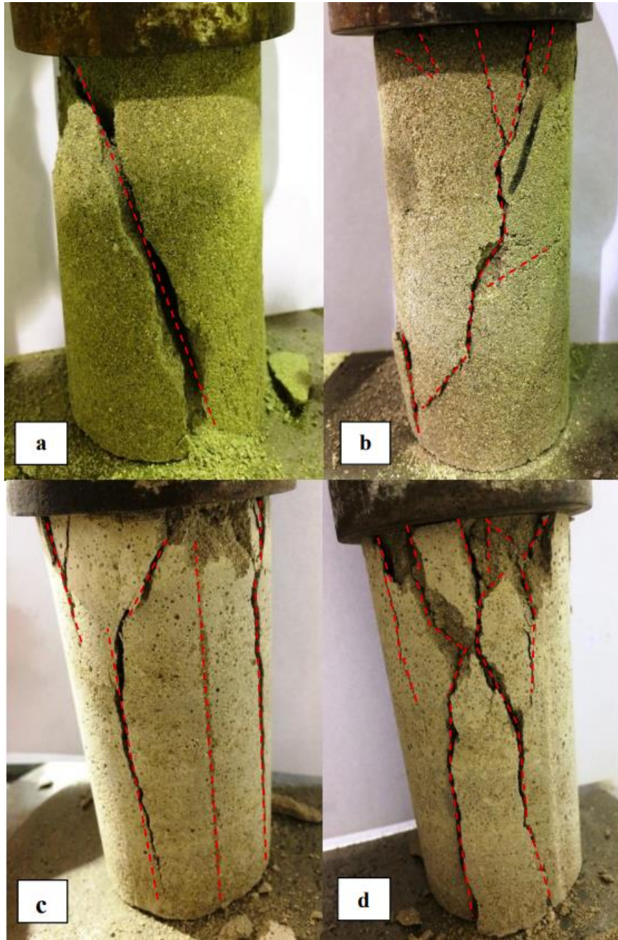
Figure 4.13: Deformation behaviour of binder-soil mixture with waste brick dust (a) 20/WBD0, (b) 20/WBD10, (c) 20/WBD20 and (d) 20/WBD30
