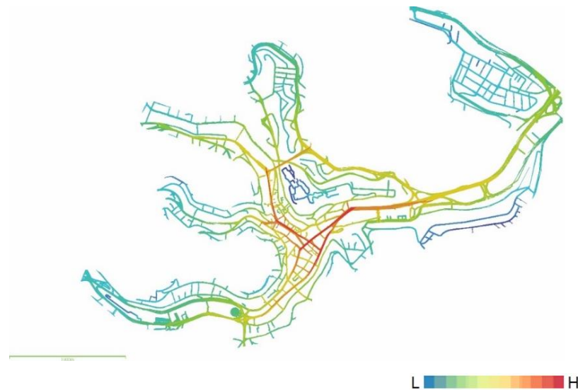
Figure 93: Axial integration map of the study area as produced by depth map.
