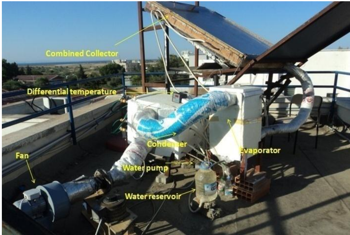
Figure 3.8: HDH Desalination system
