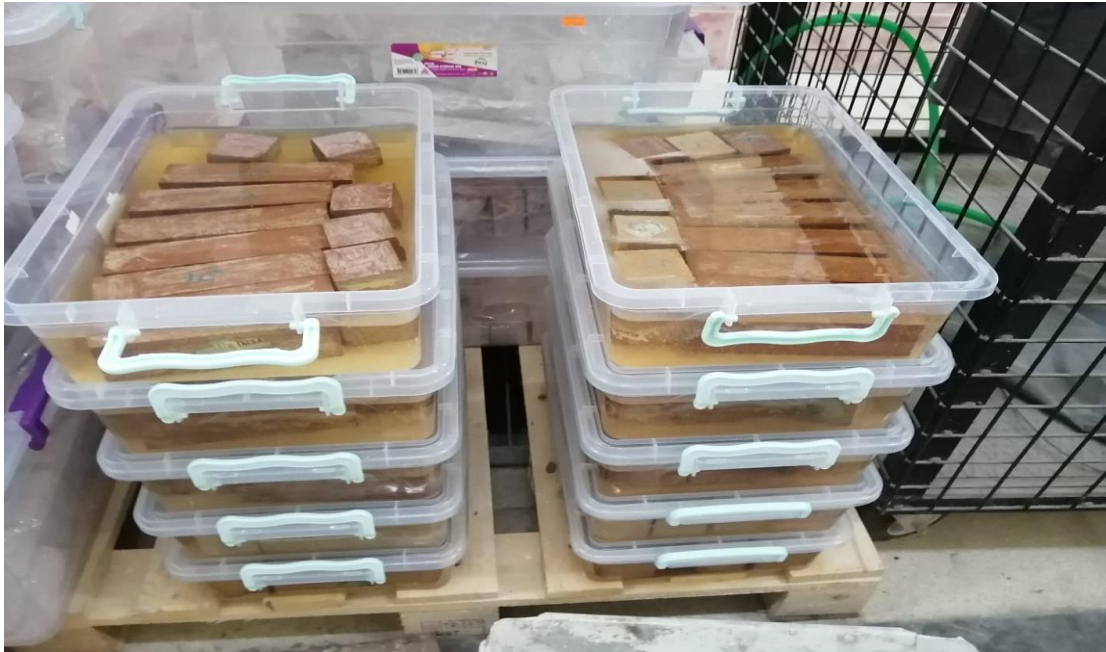
Figure 11: Geopolymer samples immersed in sulphate solution
