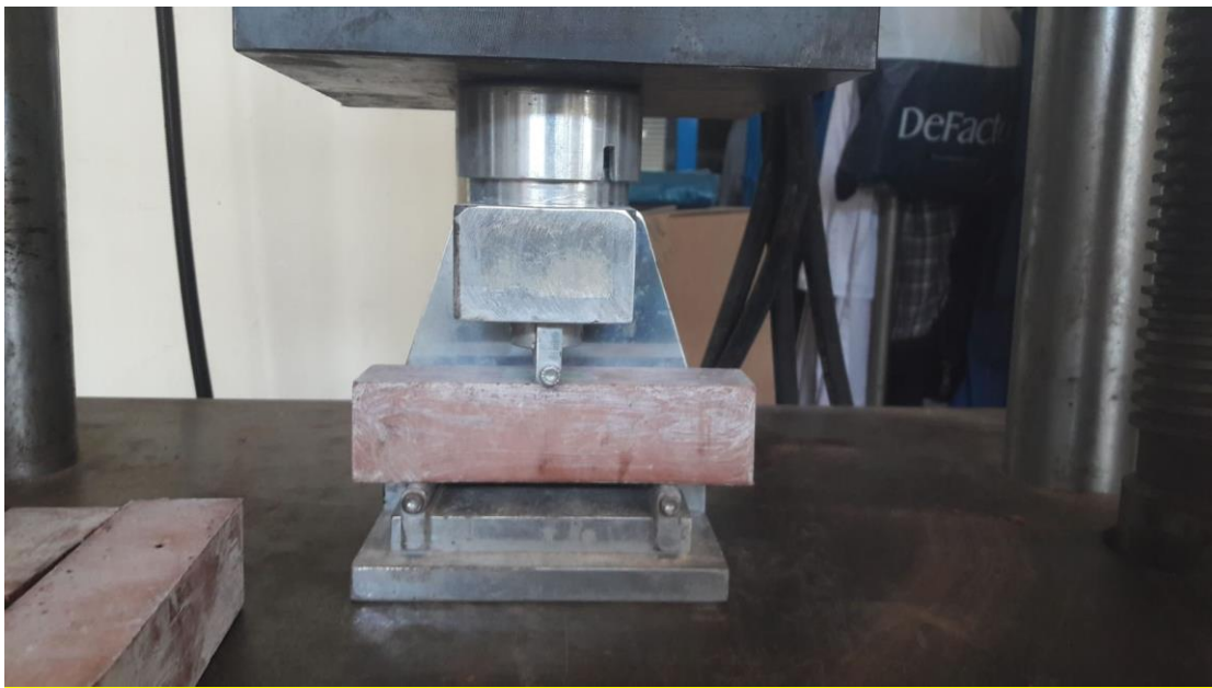
Figure 5: Flexural strength test
