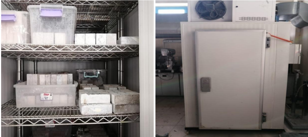
Figure 9: Freezing-thawing resistance test
