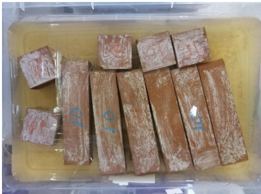
Figure 48: Specimens after magnesium sulphate effect
