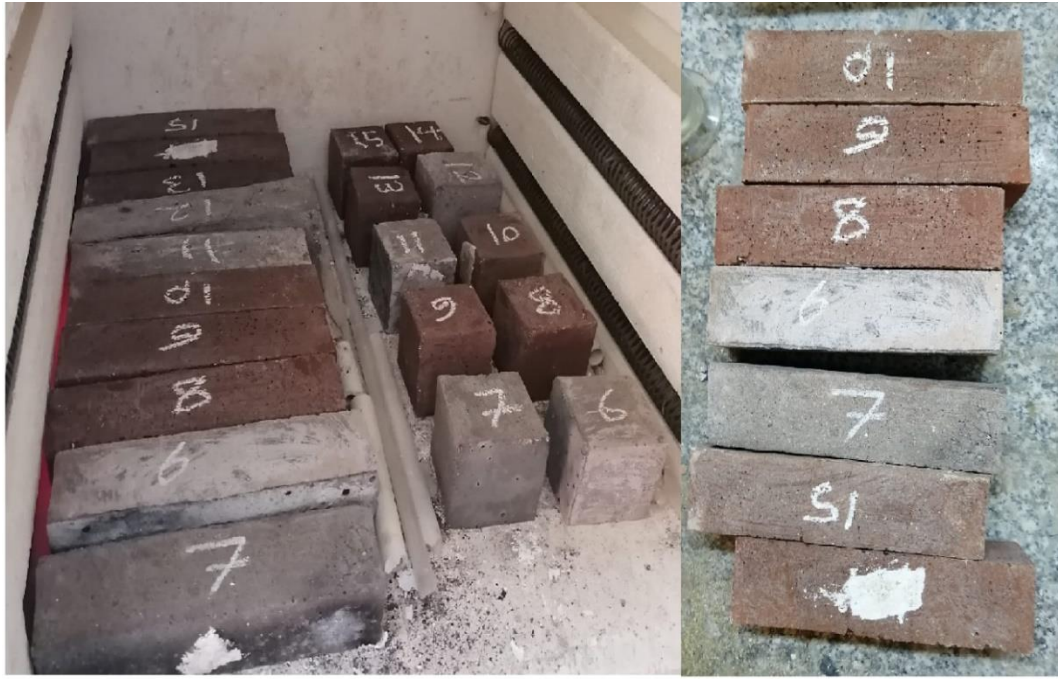
Figure 57: Specimens after 800°C effect
