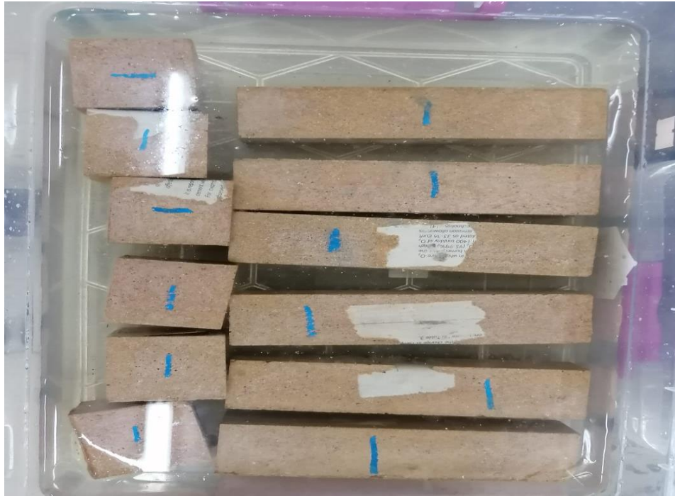
Figure 10: Geopolymer Samples Immersed in Sea Water
