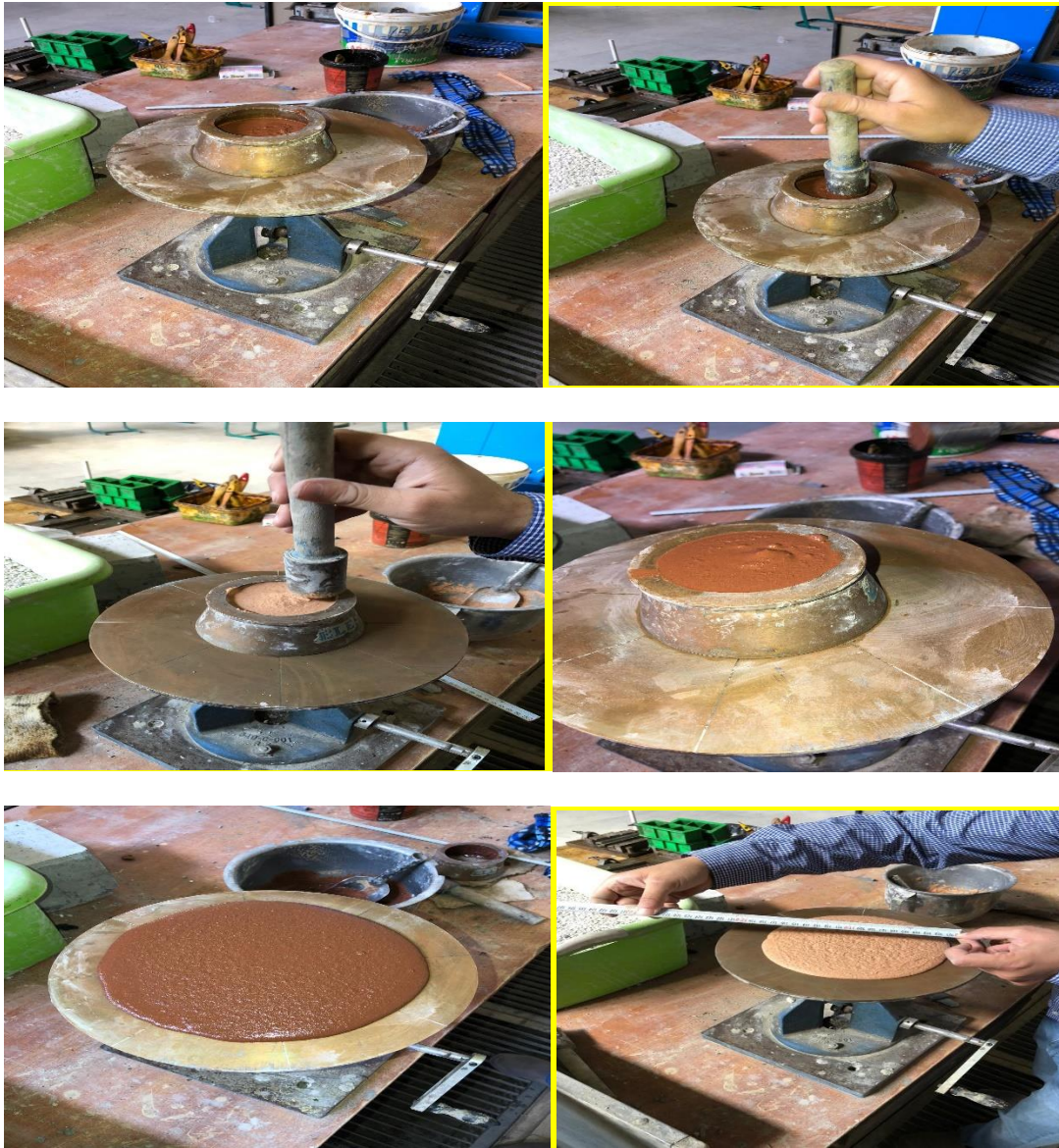
Figure 3: Steps of flow table test
