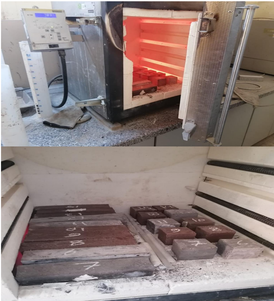
Figure 7: Elevated temperature test (800 °C)
