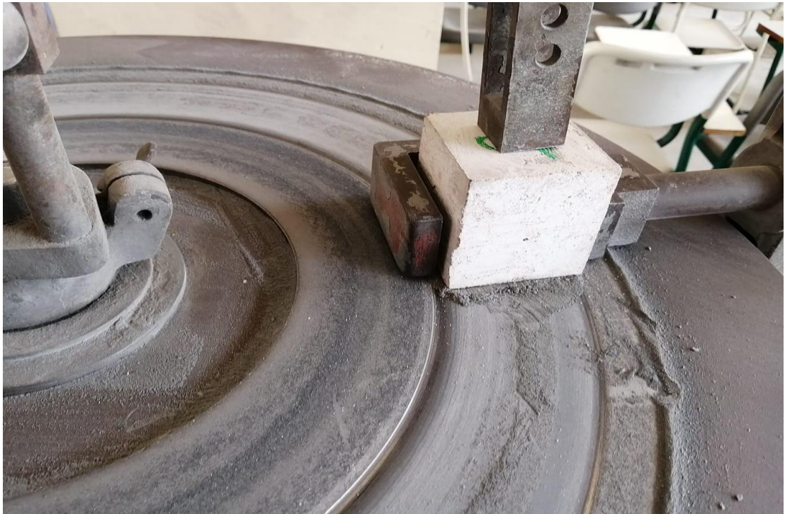
Figure 6: Abrasion resistance test
