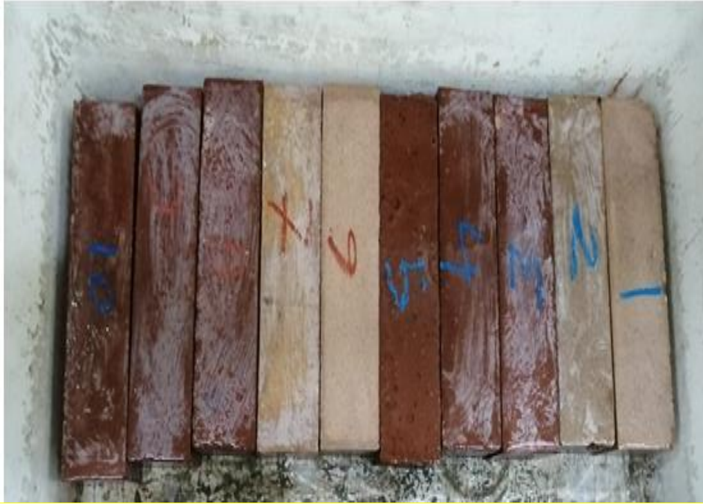
Figure 44: Specimens after seawater effect
