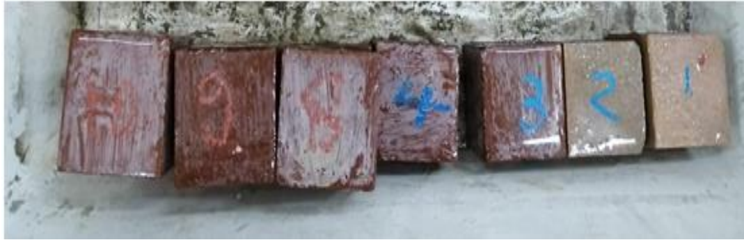
Figure 51: Specimens after freezing-thawing effect
