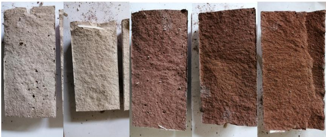
Figure 26: Samples contains GF after split tensile strength test
