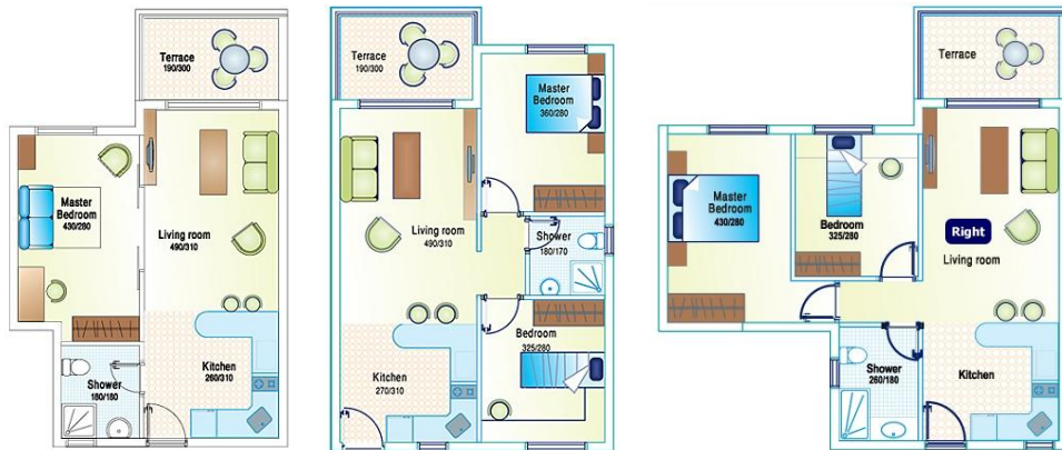
Drawing 11: Claudia block, one bedroom apartment plan 64 sqm, two bedroom apartment plan 75.5 sqm and 80 sqm Source: (Afik, 2010)
