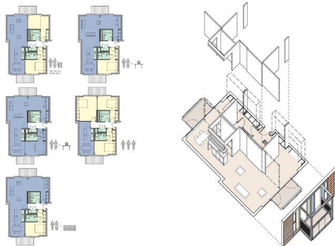
Figure 32 : Infill plans of Greenwich Millennium Village apartments in Britain Source: (Moen, Evans, Proctor, & Ogorzalek, 2002)
