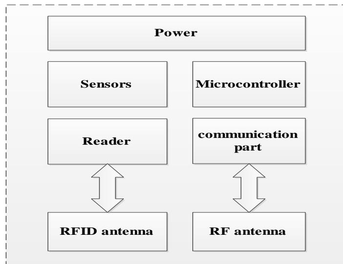
Figure 5.1: Components of Smart Node
