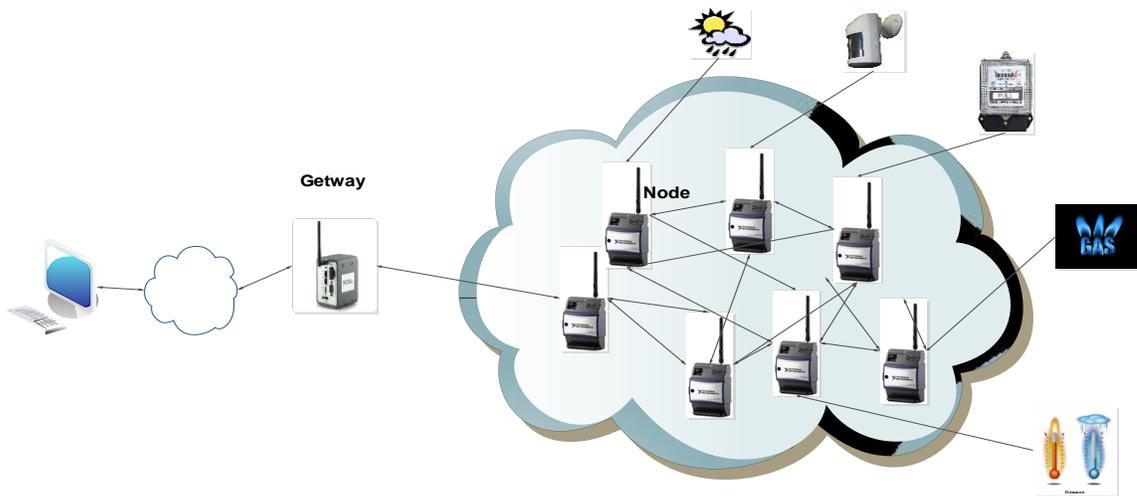
Figure 3.8: Components of Wireless Sensor Network
