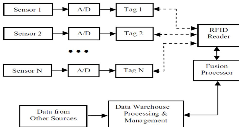
Figure 4.3: Sensor-Embedded RFID Type 2 [13]
