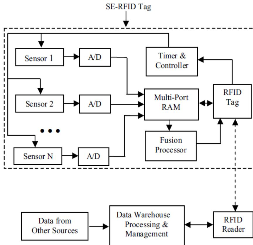
Figure 4.2: Sensor-Embedded RFID Type 1 [13]
