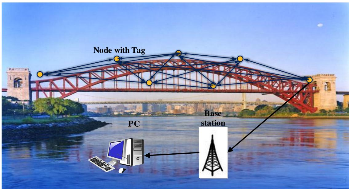
Figure 5.6: Structure of Method 2
