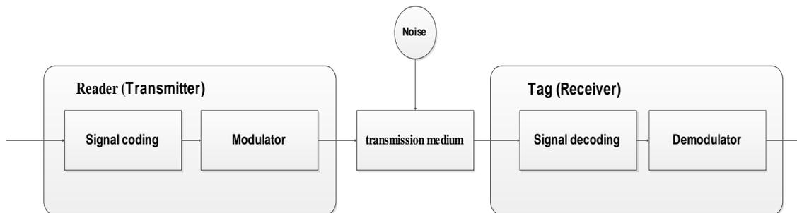
Figure 3.6: Function Blocks of Sending Data from Reader to Tag
