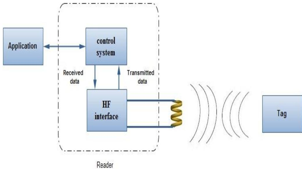
Figure 3.4: RFID Block Diagram Showing the Main Units
