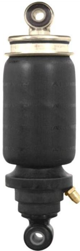
Figure 3.23: Air-spring used for experimental model [21].
