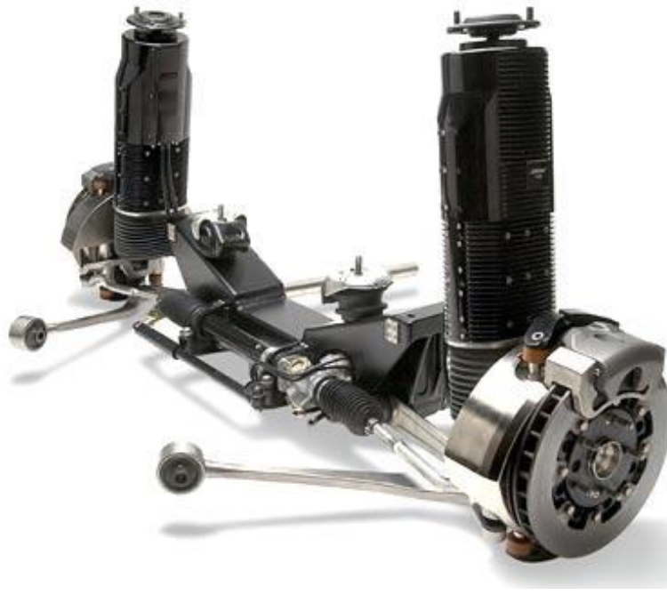
Figure 2.6: Bose suspension, an electromagnetic suspension [14].
