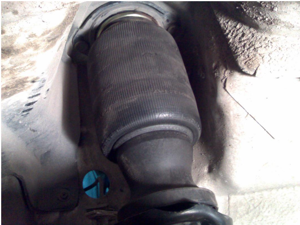
Figure 2.4: A sample of air-spring in air-suspension system.
