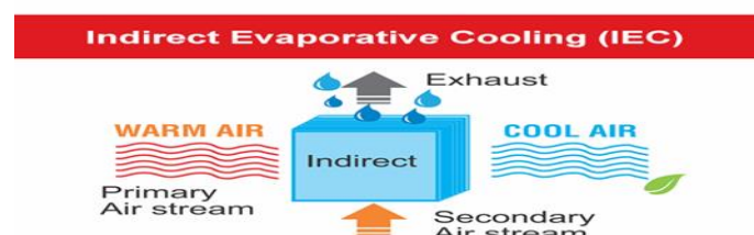
Figure 2.24: Indirect evaporative cooler Source: Alonso et al., 1998).
