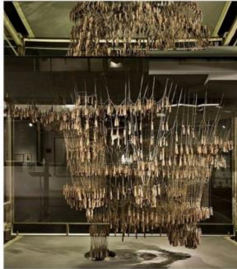
Figure 20: Analogue parametric system used by Gaudi (Assasi, 2019)
