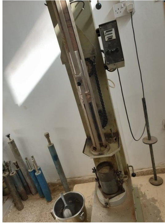
Figure 3.2: Proctor compaction apparatus used during the experiments.
