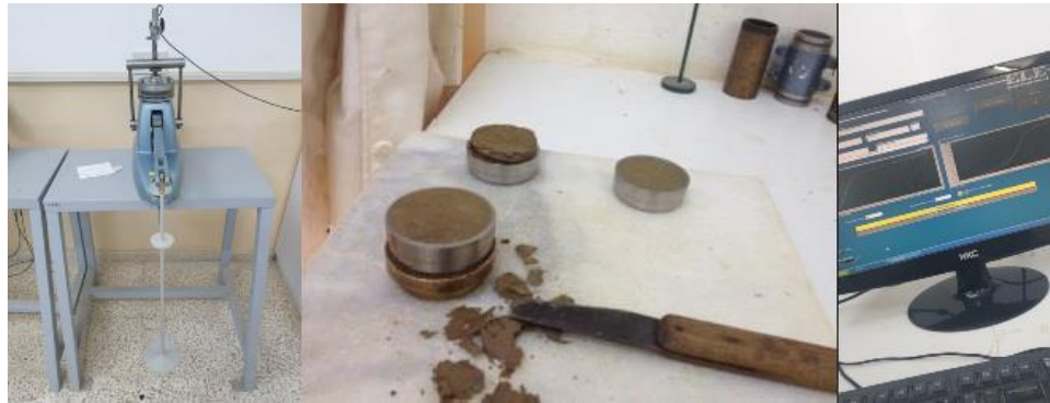
Figure 3.3: Specimen preparation for one-dimensional swell test.
