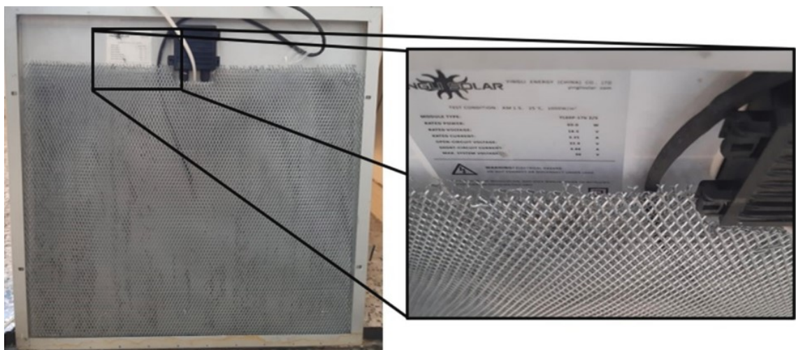
Figure 5: Porous medium integrated PV panel [64].
