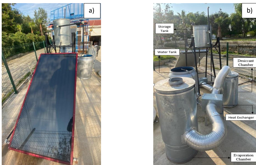
Figure 23: Designed solar assisted DAEC system (a) front view and (b) rear view
