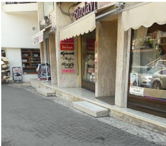
Figure 6.57: Most of the building entrances have single steps that are not available for wheelchair or scooter users
