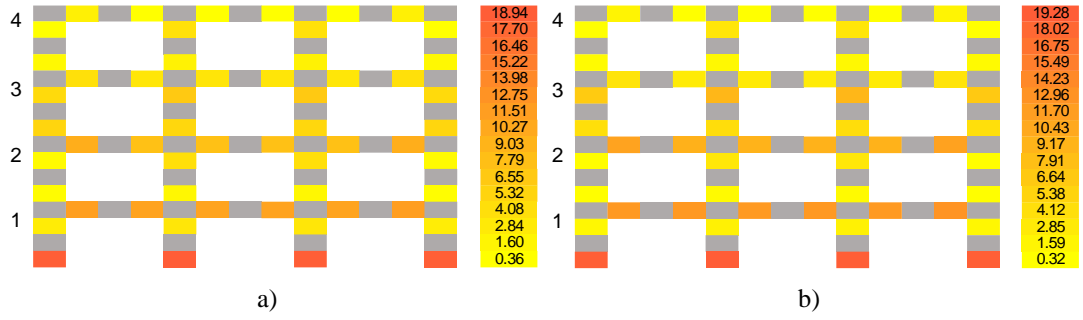
Figure 6.1: Maximum ductility demand for AS and AS preceded by MSs scaled to specific PRSD levels at collapse state (a) AS-only and (b) AS preceded by MS with PRSD=0.02 (4-story SSMF)
