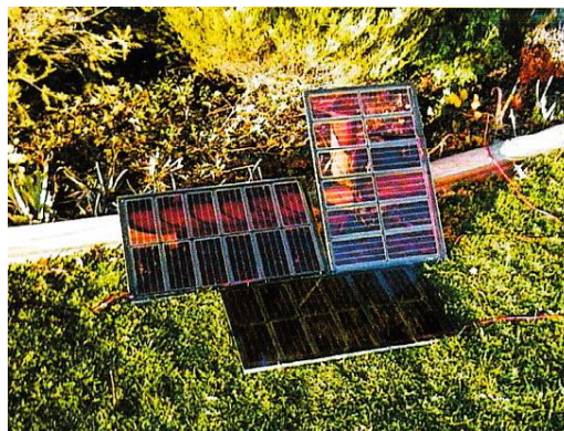
Figure 2.16: Titanium Dioxide ( \text{TiO}_2 ) Cell (Prasad et al., 2005)
