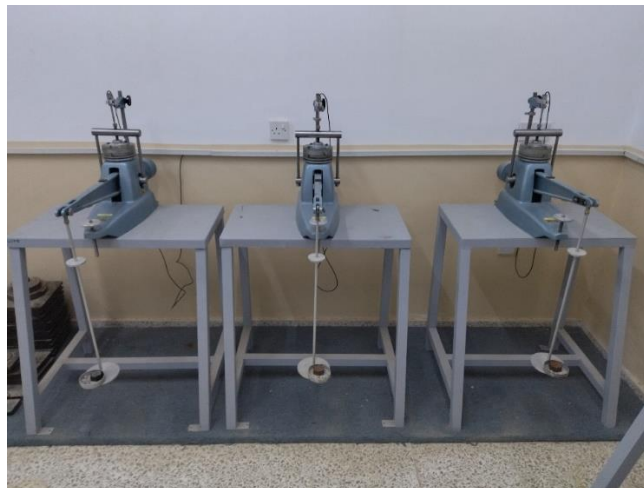
Figure 7: A standard consolidometer used in the present study
