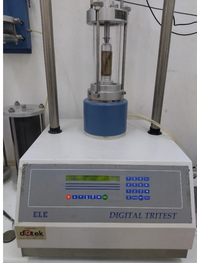
Figure 8: Unconfined compression test apparatus
