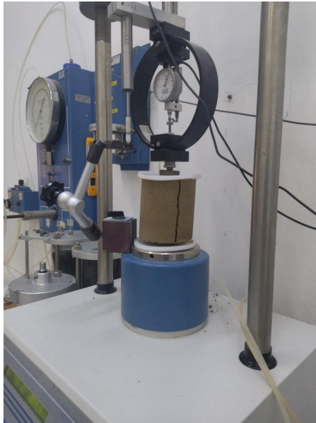
Figure 11: A set-up for double punch test
