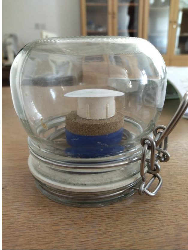
Figure 9: Prepared specimen in the glass jar for suction measurement
