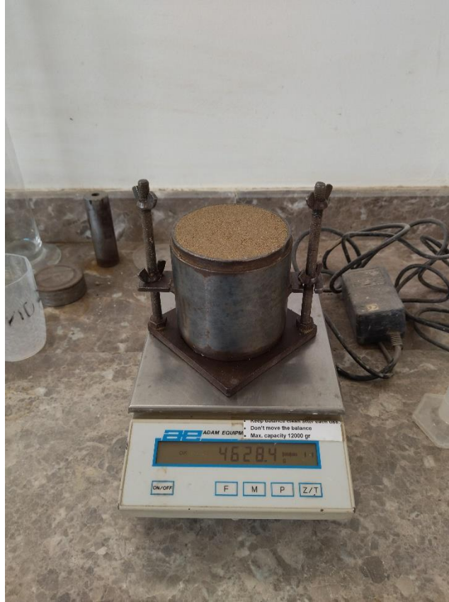
Figure 6: Compacted sand-bentonite sample after completion of compaction
