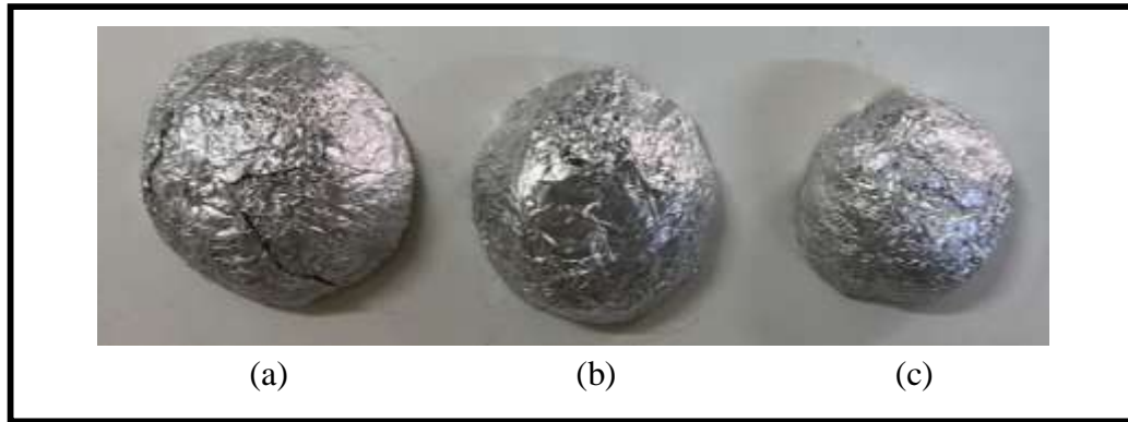
Figure 16: Molds that are used in breast phantom design. (a) 55 mm semi-spherical mold for skin, (b) 53 mm semi- spherical mold for fat, (c) 45 mm semi- spherical mold for glandular
