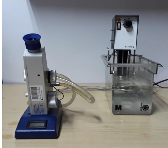
Figure 19: Experimental setup used to determine RI – temperature dependences
