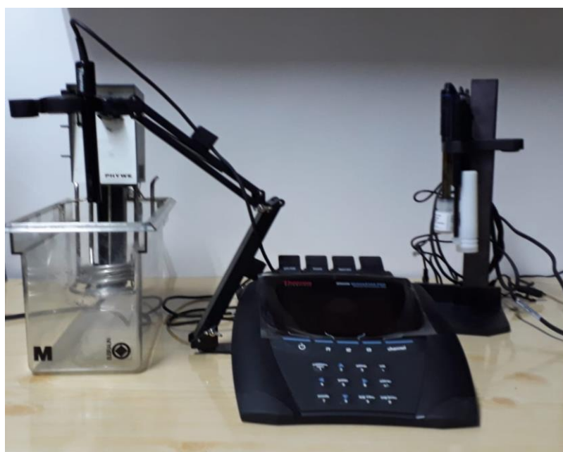
Figure 20: Experimental setup used to determine electroconductivity – temperature dependences
