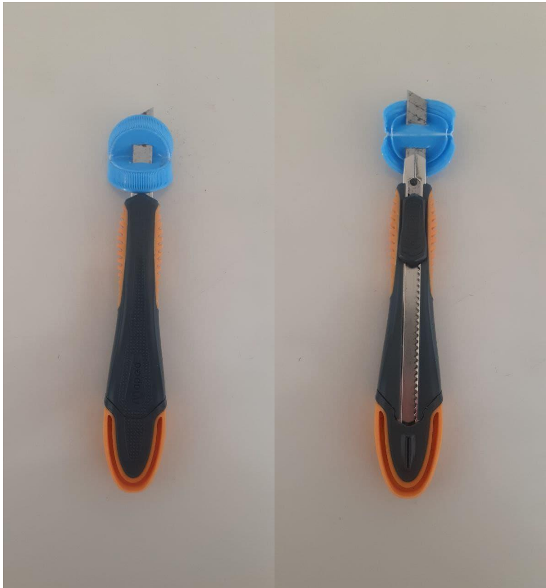
Figure 10: The tool used in order to cut the bottles into long strips
