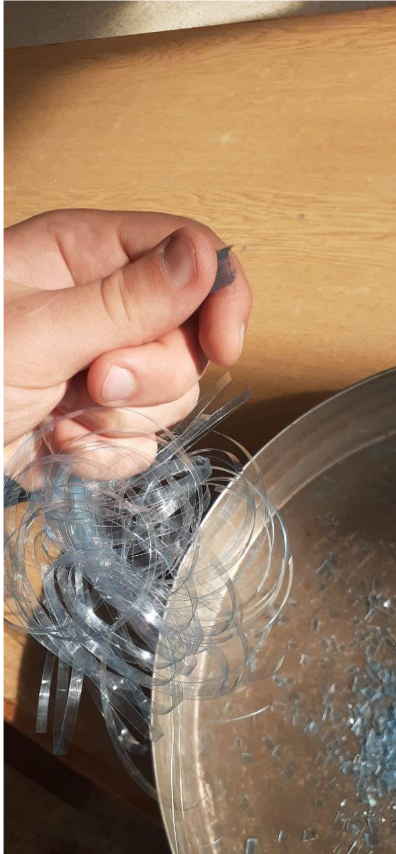
Figure 12: The hand-technique used to create 12mm×4mm long strips
