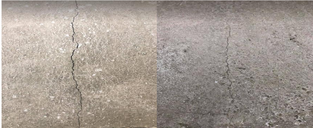
Figure 20: Failure mode of specimens during plastic shrinkage resistance test.
