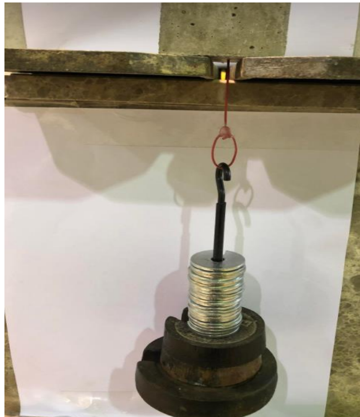
Figure 24: Pull-out resistance test apparatus.
