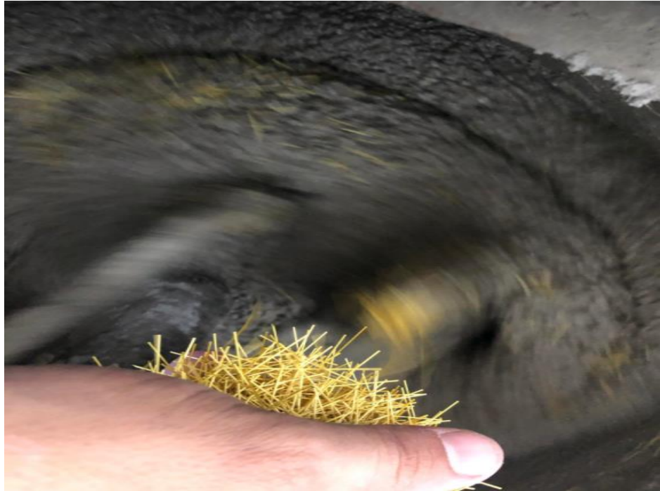
Figure 7: Utilization of recycled PET fibres to concrete mix.
