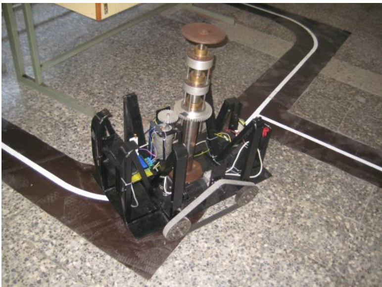
Figure 28: AGV performing curve turn to the right
