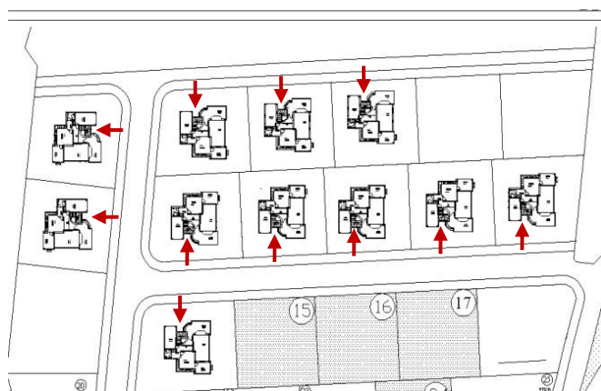
Fig 4.7. orientation of houses of type A in Mutluyaka project according to the position and entrance direction of the land
