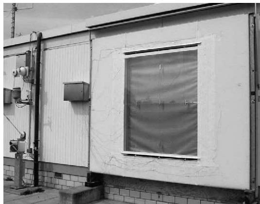
Figure 3-14: Outdoor Test Facility for Facade Elements: The test element (right) and the sensors for outside air temperature, wind speed, global and diffuse solar radiation (left) are visible (Manz, 2003: 4).
