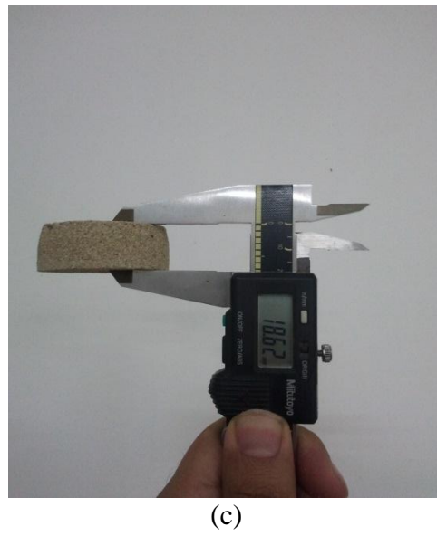
Figure 23: (a) Shrinkage test samples (b) Shrinkage diametric measurement (c) Shrinkage axial measurement
