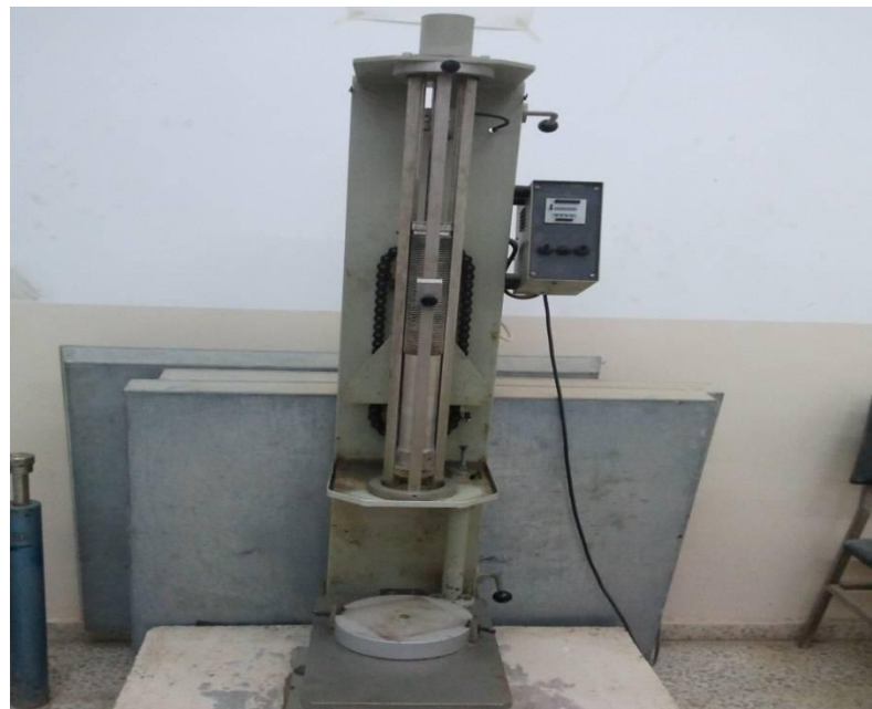
Figure 15: Automatic compaction equipment
