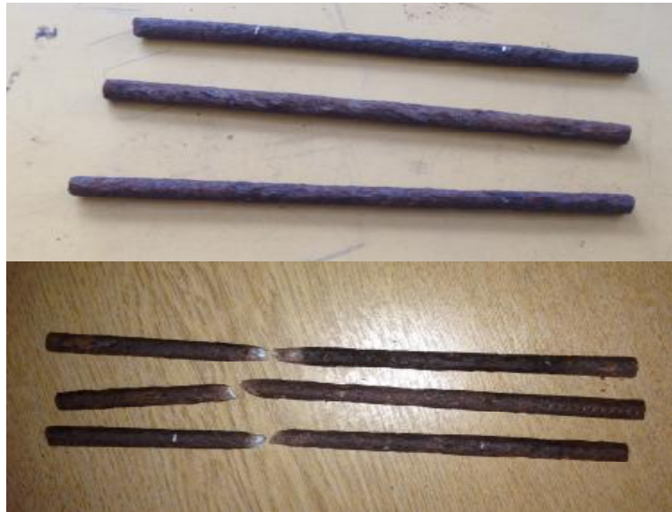
Figure 59. Three steel bar specimen before and after tension test.
