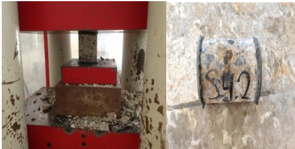
Figure 57. Compressive strength and bar steel in core sample [Materials of Construction Laboratory].
