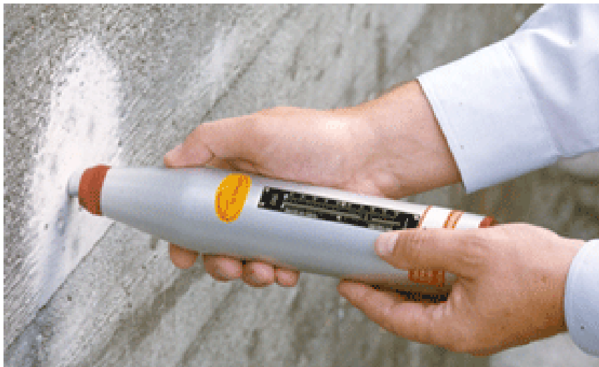
Figure 55. Schmidt hammer compressive strength taking.
