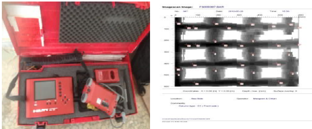
Figure 61. Ferroskan device and typical sample of ferroskan of reinforcement details.
