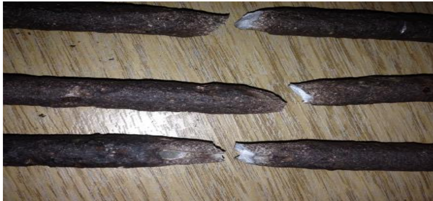
Figure 60. Specimens after tension test.
