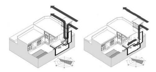
Figure 21: Diagram of Operation of Chimney in Iran (Mahmoudi, 2009)
