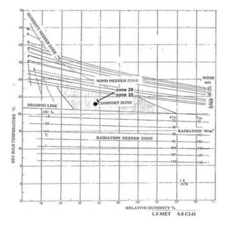
Figure 36: Bioclimatic Chart of Health Center Building in 21 March at 12:00, Zone 28, 35, East and West Office (Modified by author, Based on TAS Software data)
