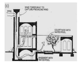
Figure 23: Way of Chimney Function for Provided Humidity (Azami, Yasrebi & Salehipoor, 2005)
