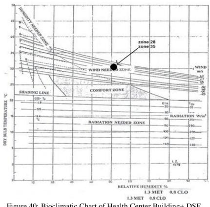
Figure 40: Bioclimatic Chart of Health Center Building+ DSF in 21 June at 12:00, Zone 28, 35, East and West Office (Modified by author, Based on TAS Software data)
