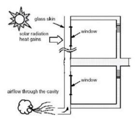
Figure 3: Heating, Ventilation and Air Flow of the Double Skin Facade (Poirazis, 2008)
