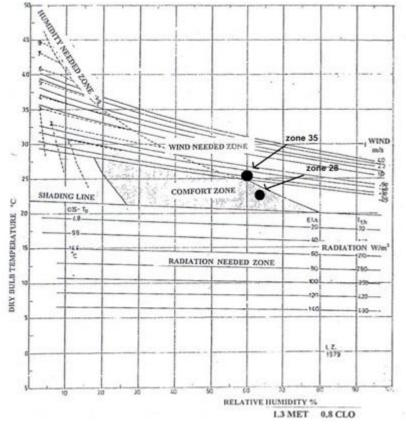
Figure 43 : Bioclimatic Chart of Health Center Building+ DSF+ Chimney in 21 March at 12:00, Zone 28, 35, East and West Office (Modified by author, Based on TAS Software data)
