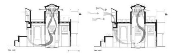
Figure 22: Diagram of Operation of Chimney in Egypt (Ficarelli, 2009)
