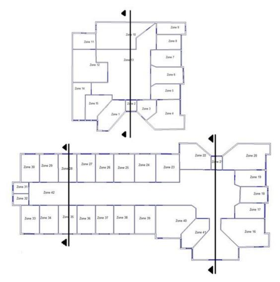
Figure 29: Health Center Zones in TAS Software (Underground and Ground Floor Plan (Drawn by author, through the given plans by Architecture Department, 2013)
