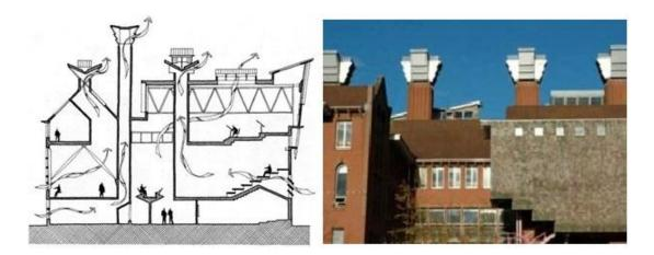
Figure 24: Ventilation by Natural Wind Flow (Kleiven, 2003)
