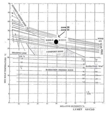
Figure 44: Bioclimatic Chart of Health Center Building+ DSF+ Chimney in 21 June at 12:00, Zone 28, 35, East and West Office (Modified by author, Based on TAS Software data)
