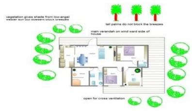
Figure 17: Building Plan in Hot and Humid Climate (Fordham, 2000)
