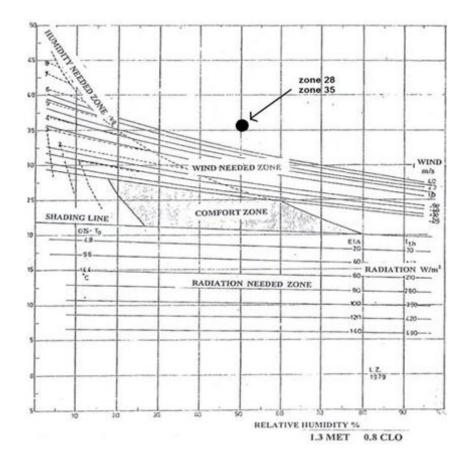
Figure 41: Bioclimatic Chart of Health Center Building+ DSF in 21 September at 12:00, Zone 28, 35, East and West Office (Modified by author, Based on TAS Software data)
