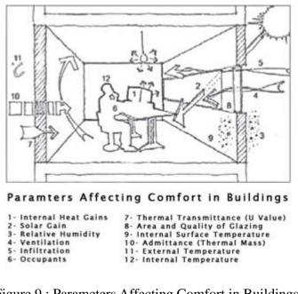
Figure 9 : Parameters Affecting Comfort in Buildings (Allard, 1988)
