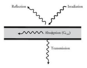
Figure 2: Reflection, Absorption and Transmission of Solar Radiation of Glass (Poirazis, 2008)
