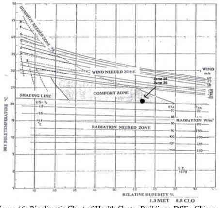
Figure 46: Bioclimatic Chart of Health Center Building+ DSF+ Chimney in 21 December at 12:00, Zone28, 35, East and West Office (Modified by author, Based on TAS Software data)
