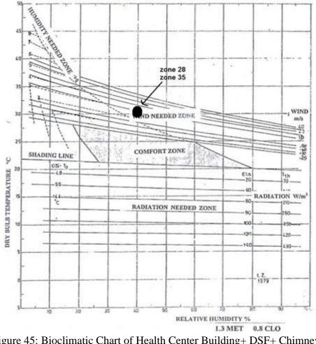
Figure 45: Bioclimatic Chart of Health Center Building+ DSF+ Chimney in 21 September at 12:00, Zone 28, 35, East and West Office (Modified by author, Based on TAS Software data)
