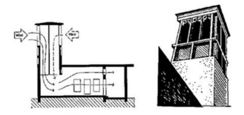
Figure 20: Vertical Ventilation Increases the Thermal Comfort Situation (Mahmoudi, 2009)
