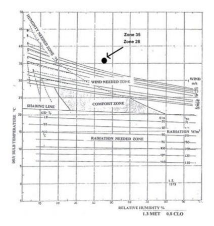
Figure 37: Bioclimatic Chart of Health Center Building in 21 June at 12:00, Zone 28, 35, East and West Office (Modified by author, Based on TAS Software data)
