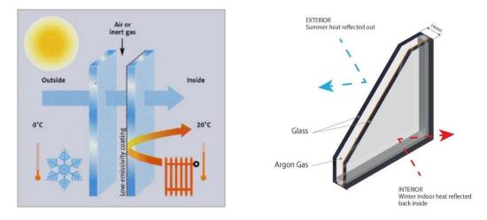
Figure 1: Double Glazing Window. (Knaack, Klein, Bilow and Auer, 2007)
