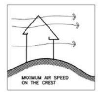
Figure 16: Maximum Air Speed on the High Level (Fordham, M, 2000)
